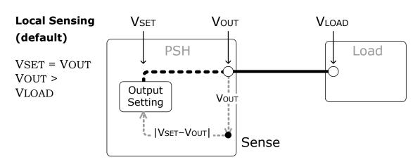
The sense terminal is internally connected to the PSH output terminal. The delta between the voltage setting level (VSET) and the actual output level (VOUT) is compensated. The load terminal voltage (VLOAD) might become lower than the output due to cable loss.
