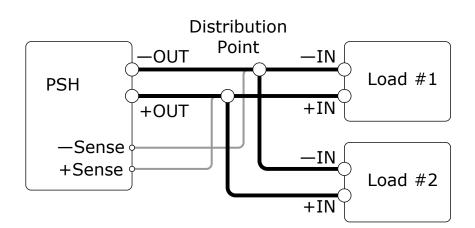
Create a distribution point between PSH and the loads. PSH compensates the cable loss up to the distribution point.
