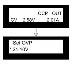
2. Press the F/C key to move the underline before or after the decimal point.
