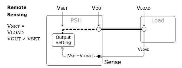
The sense terminal is connected to the load input terminal. The delta between the voltage setting level (VSET) and the actual load voltage (VLOAD) is compensated. The output voltage (VOUT) might become higher than the setting due to the compensation.
