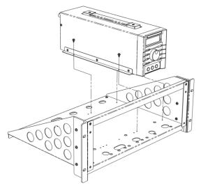
Fix the front panel and the handle to the main bracket using M4 screws.
