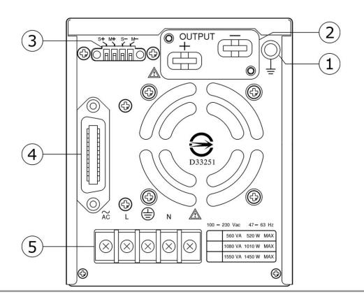
1 Ground Terminal Connect the output line shield (page25) and the remote sensing line shield (page33).
