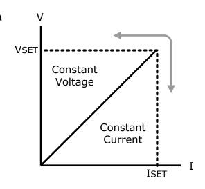
VSET = Output Voltage setting ISET = Output Current setting
