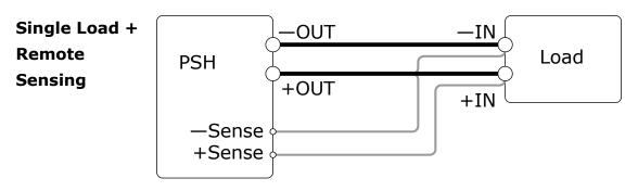
Connect both the output wire and the remote sensing wire to the load.
