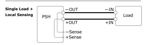
Connect the output wire to the load and the sense terminal to the PSH local output monitor.
