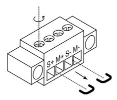
2. Screw wires to the sense (S) side.
