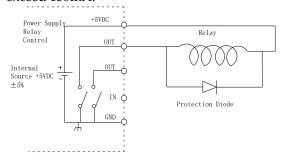
Warning: Do not short the 5VDC terminal to the chasis, earth or to the control port GND, otherwise it may damage the unit.
