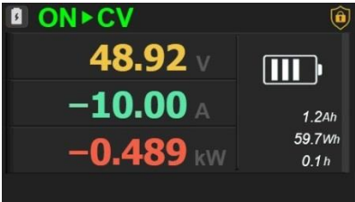
Figure 3-10-6 Battery discharging running interface
