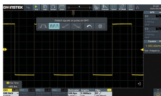
The AUTOSET Button Automatically Identifies Waveforms
