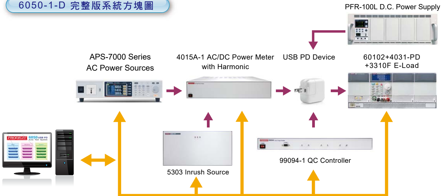
6050-1-D Single Channel Test System Configuration
