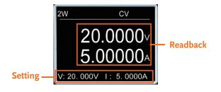
The set value and the actual readback value after the output is turned on can be displayed directly on the screen at the same time.
