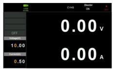
3. Repeatedly press the Voltage knob until the target digit is highlighted. This will allow the voltage to be edited in 0.01 volt steps.
