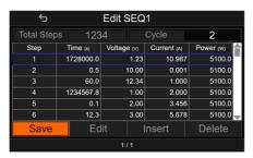
9. The message box "Access ..." will appear, analyzing the entire sequence process. Since the editing is done locally, it only needs to check if "Loop" and "Endloop" are paired correctly and ensure there are no recursions. If everything is correct, the data will be saved, and the message box will close.
