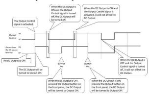
When the Output OFF signal is turned off, the relationship between the Output ON signal and the Output Control signal is as follows.
