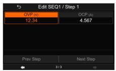
OVP: Set the over-voltage protection value. OCP: Set the over-current protection value.
