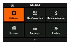
2. Press the Voltage knob to enter the Settings Page and rotate the Voltage knob to choose the "Protection" icon.
