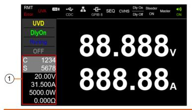
Block of Function Setting Displays the Setting of Function and status. (Sequence, SAS and other simulation)
