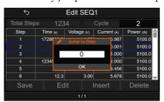
7. In the "Jump to Step" dialog box, pressing the Voltage Knob will directly jump to "Edit".
