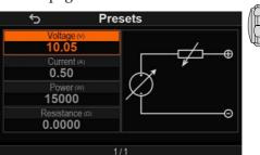
4. Press the Voltage knob, and it will be a place that can use the number pad to set the value directly.
