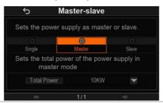
Master: The user can set the total power of up to 150 kW.
