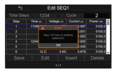
11. In the "Edit SEQ1" menu, rotate the Voltage Knob to "Edit" and press the Voltage Knob. This will enter the "Edit SEQ1 / Step1" first page setting menu.
