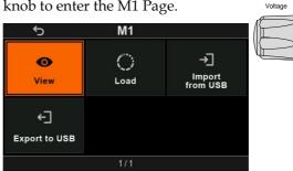
Rotate the Voltage knob to choose the "Load" icon. And Press the Voltage knob to complete loading memory.
