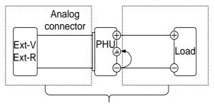
(······) Insulation capacity ≥ voltage of power supply with respect to ground
