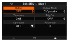
Output: Control "Output OFF" and "Output ON".
