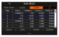
6. Press the Current Knob to bring up the "Jump to Step" dialog box, allowing you to immediately jump to the entered Step.
