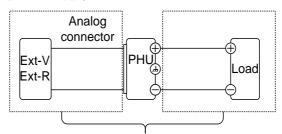
(-----) Insulation capacity ≥ isolation voltage of power supply
