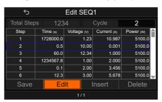
8. In the "Edit SEQ1" menu, rotate the Voltage Knob to "Save" and press the Voltage Knob.
