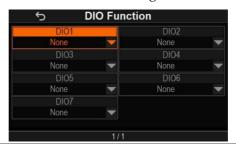
Input mode Output OFF, Output ON, Output Control, Clear Alarm, Load M1, Load M2, Load M3
