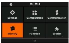
3. Press the Voltage knob to enter the Memory Page and rotate the Voltage knob to choose the memory slots.(M1, M2, M3)
