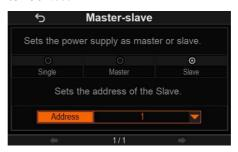
Slave: The user can set Slave units numbered from 1 to 10.
