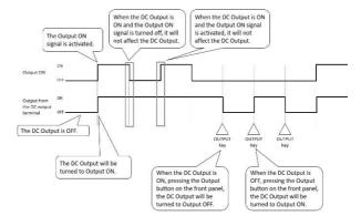
When the Output OFF signal is turned off, the relationship between the Output Control signal and the Output button operation is as follows.
