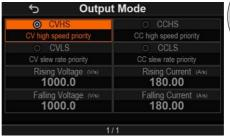
4. Users can choose the Output Mode by rotating the Voltage knob. Press the Voltage knob to complete selection.
