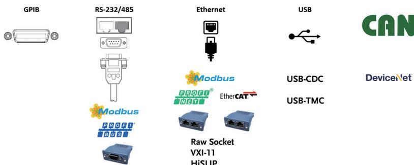
PHU provides a variety of embedded industrial interface options to meet user needs, eliminating the need for users to prepare additional interfaces.
