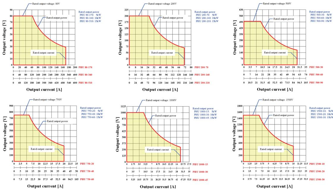
This feature enables the power supply to automatically adapt to higher output voltages when there is a smaller current or handle higher currents when there is a lower voltage. It allows the use of a single source to address multiple voltage and current combinations.
