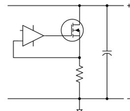
The bleeder circuit is a power supply circuit designed to discharge the electric charge stored in the power supply filter capacitors when the equipment is turned OFF, primarily for safety reasons to protect the DUT.
