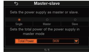
The unique APC (Adaptive Parallel Connection) feature offers adaptability in parallel connection, allowing users to make the best choice according to their needs. For instance, users can opt for a 15 kW model and a 10 kW model, to combine both to reach a 25 kW capacity within their budget constraints. Up to 10 PHU units can be connected to reach 150 kW without the need for additional power distribution for control.
