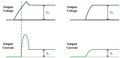
The PHU-Series has CV and CC priority modes. The CC priority mode can prevent inrush current and surge voltage from occurring at turn-on to protect DUT.
