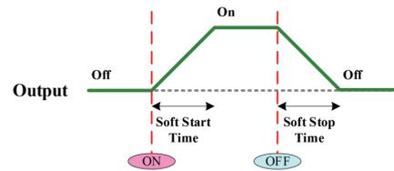
The default voltage (or current) rising speed when starting/stopping the output is set as the highest speed. PHU provides the function for the user to set the speed per their request for applications.
