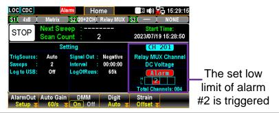
6. Also, the alarm details will be saved in the memory when the set alarm occurs for select channel during a scan course. Press the *View* key on the front panel to view the info of triggered alarm. Refer to page 120 for details of View menu.
