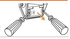
2. The fuse socket appears. The "240" symbol within the hole on fuse socket indicates the line voltage is positioned as 240V.
