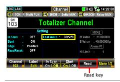
Press the F6 (More 1/2) key to forward to the next page where the F2 (ReadReset) key allows user to turn On or Off automatic reset on totalizer count, and the F3 (Edge) key allows user to specify whether the totalizer channel should count on the rising (Pos) edge or falling (Neg) edge.
