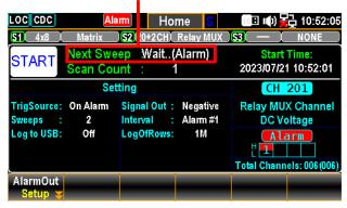
F2 (Time) key When Time of TrigSource is selected, press the key to specify a to set interval time interval.
