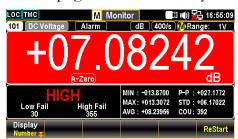
Values Left Sec. The numbers of High and Low limits exceeding are shown individually. Right Sec. The values, which based on dB calculation, identical to STAT page are well displayed.
