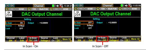
Press the F4 (Source) key to toggle between Voltage and Current, which indicates that the selected DAC channel outputs in either Voltage or Current mode.
