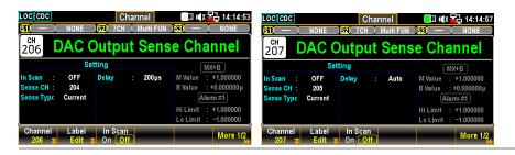
Press the F3 (In Scan) key to designate if the select channel is included in (On) or excluded from (Off) the scan list.
