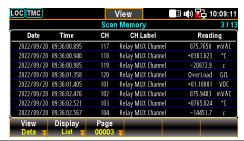
3. The list mode displays Date, Time, Channel, Channel Label (naming by user) and reading of each measured data from a scan course.
