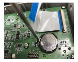
5. Use fingers to take the battery out off the compartment with ease.
