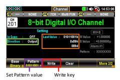
Press the F4 (Clear) key to define the set Pattern back to zero "0". Repeat pressing the F3 (Write) key to overwrite newly set output Pattern.
