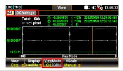
3. When the "GRH" is selected for *ViewMode* (F3) key, scroll the *knob* key to navigate through scanned counts. If pressing *knob* key, the maximum counts moving by scrolling *knob* key per time will be changed.
