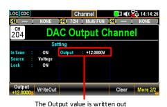
Press the F5 (Clear) key to restore the set Output value back to zero "0". Repeat pressing the F2 (WriteOut) key to overwrite newly set Output value.
