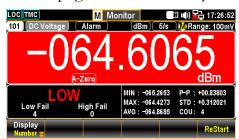
Values Left Sec. The numbers of High and Low limits exceeding are shown individually. Right Sec. The values, which based on dBm calculation, identical to STAT page are well displayed.
