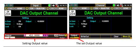
The F2 (WriteOut) key allows user to write in the set Output value to the Output field, which is located in the Setting area on display.
