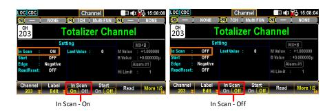
Press the F4 (Start) key to toggle between On and Off, which indicates that it starts to count on the totalizer channel or it stops to count on the totalizer channel.
