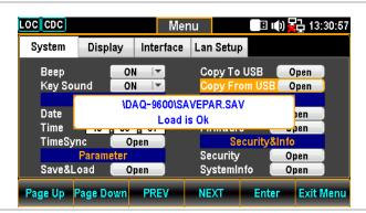
6. The prompt message indicates the selected parameters is loaded from the connected USB disk to DAQ-9600.
