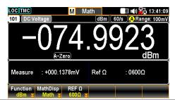
Values -074.9923 dBm Indicates the latest dBm value Measure Indicates the originally measured Voltage value Ref $\Omega$  Indicates the defined ref  $\Omega$  value
