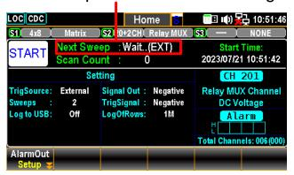
On Alarm It indicates a sweep starts when an alarm is detected from the set channel. Press the On Alarm (F2) key to specify which alarm (1-4) is used to report on the select channel.
