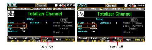
Press the F5 (Read) key to fetch the latest count of totalizer. Please note that since number of count(s) doesn't refresh on the display automatically, pressing the Read key to read count once each time.
