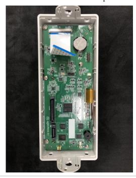
8. Connect every cable and cord in need and reassemble the instrument in proper order. The procedure of battery replacement is completed.
