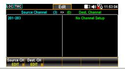
4. Use *knob* key to navigate channels followed by pressing *Select* or *Select All* to select destination channels. Press *Cancel* or *Clear All* to deselect channels. Press *OK* to confirm selection. Press *Exit* to leave the page without saving the selection.
