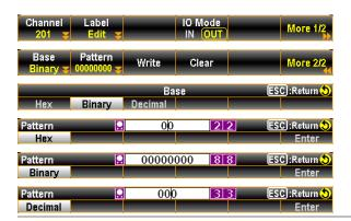
Press the F3 (Write) key to output the set Pattern on the selected channel of digital output. The Last Value of Setting area on display will be updated accordingly.
