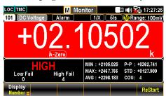
Values Left Sec. The numbers of High and Low limits exceeding are shown individually. Right Sec. The values, which based on 1/Xcalculation, identical to STAT page are well displayed.
