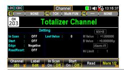
Press the F3 (In Scan) key to designate if the select channel is included in (On) or excluded from (Off) the scan list.
