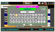
6. Press the F4 (OK) or the Knob key to confirm the input words.
