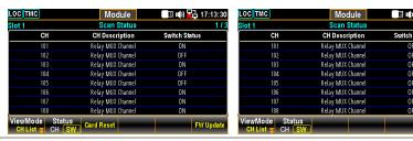
4. When user intends to carry out firmware update for installed module, press the *FW Update* (F6) key to perform update process. The prompt message pops up and user can press *Yes* (F1) to carry on the update.
