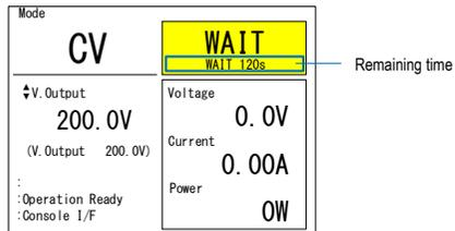
This device has an inrush current prevention circuit on the AC side. Because this circuit requires cooling, it is necessary to leave an interval for a certain period after the last use. Cooling time is up the WAIT status in the following cases.
