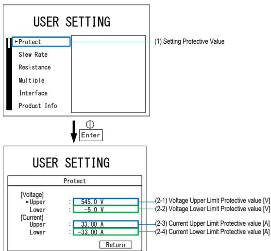
2. Set each protection value. Press the knob to display the cursor. Use the SHIFT key to select the digit, set the protection value, and press the knob to determine it.
