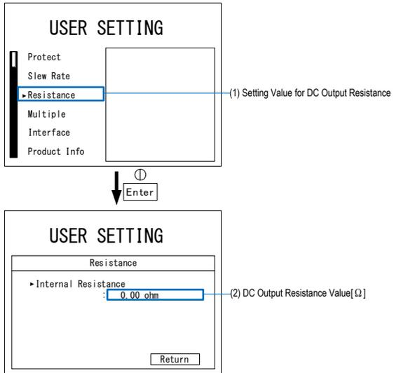
2. Press the knob to display the cursor. Select the digit with the SHIFT key, set the DC output resistance value, and press the knob to determine it.
