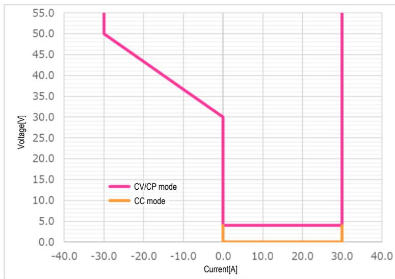
The current in the AC → DC direction is assumed to be positive. During series-parallel operation, the number of units is multiplied by the same value.
