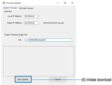
7. Receiving update firmware from PC. Never turn off the power of this equipment during reception.
