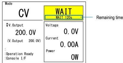
This device has an inrush current prevention circuit on the AC side. Because this circuit requires cooling, it is necessary to leave an interval for a certain period after the last use. Cooling time is up the WAIT status in the following cases.
