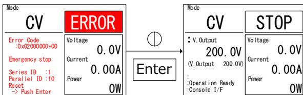
6. After the emergency stop, the screen is remained to the ERROR window.
