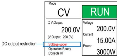
When only one DC output limit status is used, the output limit name in the table below is displayed. When multiple occurrences occur at the same time, they are displayed as hexadecimal numbers in the left-most bit arrangement.
