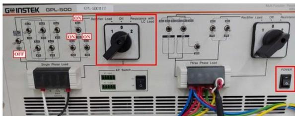
7. After setting, launch PSW output via SAS program followed by enabling APS-300 output and finally turn on the switch of PEK-510.
