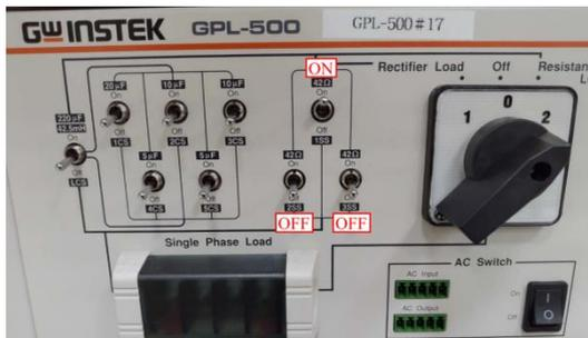
The figure 4.12 shows that when GPL-500 is set as light-load mode, VO RMS voltage is 0.507V (40.89V in actual value), and IO RMS voltage is 0.772V (0.97A in actual value).
