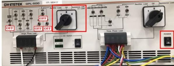
8. After setting up, turn on PSW output via SAS programm and enable APS-300 output followed by turning on the switch of PEK-510.
