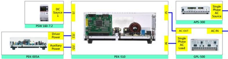
Figure 8.5 Experiment 8 wiring figure
