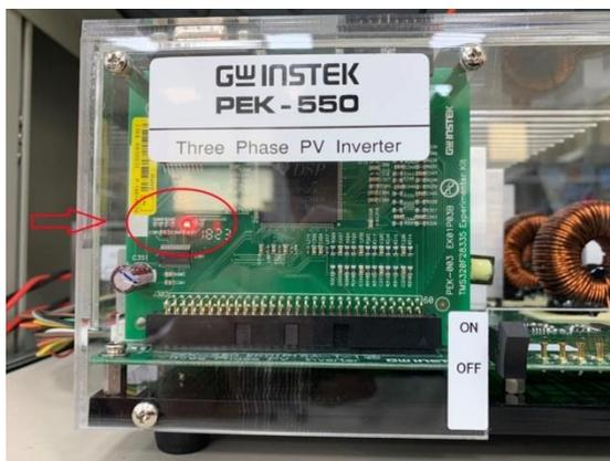
2. Connect one end of RS232 cable to PC, and the other end to the RS232 connector of PEK module.
