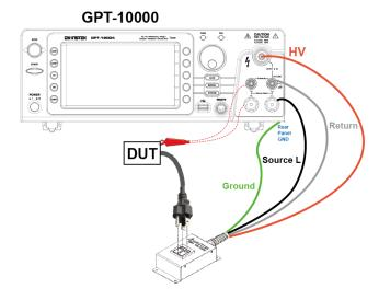
Connection with GPT-10000 diagram in Continuity test
