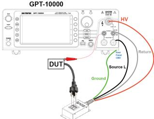
1. Connect the red wire to the High Voltage terminal HIGH VOLTAGE Terminal of the GPT series.
