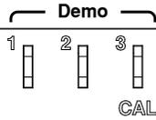
The Demo outputs are multifunction outputs that can be configured for probe compensation, as a trigger output or as a basic waveform generator for demonstration purposes. (FM signal, UART, I<sup>2</sup>C, SPI).
