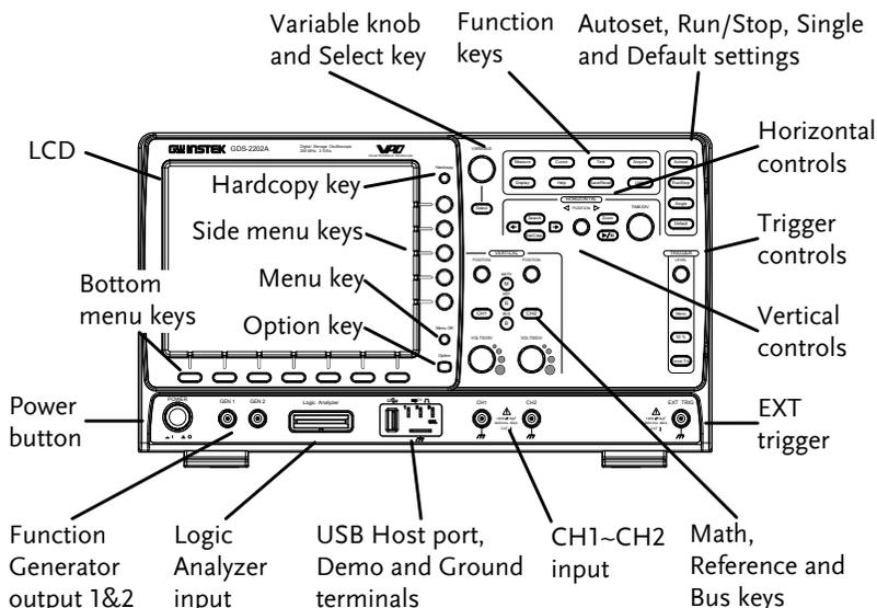
**LCD Display**      8" SVGA TFT color LCD. 800 x 600 resolution, wide angle view display.
