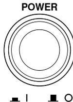
Used to turn the power on/off.
