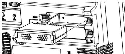
4. Slide the tabs back into the lock position.
