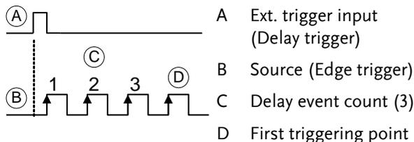
Delay trigger example (by time)
