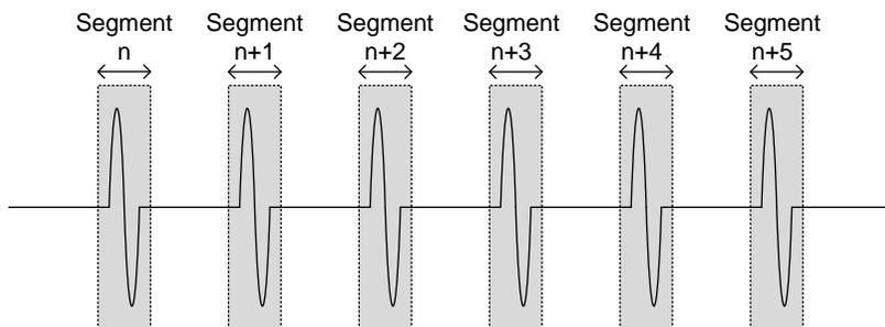
As shown below, the memory is divided into segments to increase the number of events that can be effectively captured with the same acquisition memory. Also notice that the scope doesn't need to rearm the trigger between each segment, this makes the segmented memory function especially useful for high speed signals. The time between each segment is also recorded so that accurate signal timing can also be measured.
