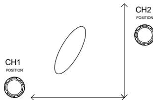
The horizontal position knob and Time/Div knob can still be used under the XY mode.
