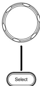
The Variable knob is used to increase/decrease values or to move between parameters.
