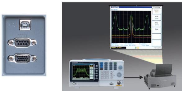
The USB host interface on GSP-730 front panel allows the measuring diagrams to be saved in the memory stick. The USB Device and RS232 interfaces on the rear panel are capable of connecting with PC for remote control. VGA output can transfer
