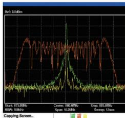
The GSP-730 can illustrate a signal with three colors simultaneously under various display modes, including Clear/Write, Max-Peak Hold, Min-Peak Hold, View, Blank and Average. Other useful trace functions such as trace math operations are also accomplishable.
