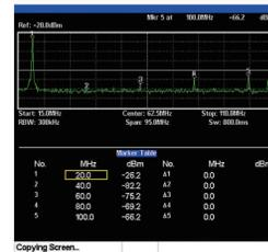
Five Markers can be used to obtain the measurement readings of specified points. Each marker has a counterpart  $\Delta$ Marker, the amplitude difference can be measured and indicated by setting the frequency of marker and the interval frequency of  $\Delta$ Marker between two signals. While several pairs of Markers are used for marking more than one pair of signals at the same time, the Marker Table can be turned on and it can process all the tests and demonstrate the reading figures.
