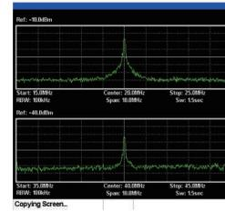
Under Split Window Display Mode, the monitor will display two independent screens, which can respectively have separated settings. For instance, if processing the test between fundamental and harmonic signals, the separated screens can respectively set at different frequencies at the same time in order to process the measurement.
