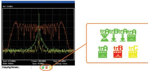
The intuitive icons help user grasp the current setting conditions all the time. As all status icons are clearly shown at the corner of the screen, there is no need to worry about the unknown settings, which may cause confusion and lead to measurement errors.
