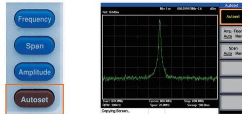
The Autoset function automatically captures the signal and configures an appropriate setting for the optimum spectrum display at just one press of the button. With the Autoset function, using a spectrum analyzer like GSP-730 is no longer an annoying and complicated task.
