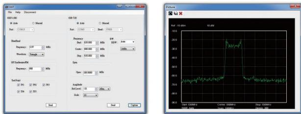
The dedicated PC software, Primary RF, is provided to support the remote control of GSP-730 and GRF-1300 simultaneously. The control includes base band signal waveform, frequency and RF signal frequency for GRF-1300 and Frequency, Span, Amplitude, RBW and spectrum transferring of GSP-730.
