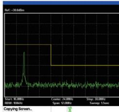
This function may run the "Pass" and "Fail" inspection with efficiency. Firstly, a limit line or upper and lower limit lines should be edited as the judgment criterion, then the LCD will display "Pass" or "Fail" according to whether the input signal meets the condition defined by the limit lines to indicate the examined outcome.
