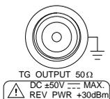
The Tracking Generator (TG) output source.
