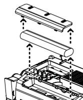
2. Replace the battery with the same type and specification.
