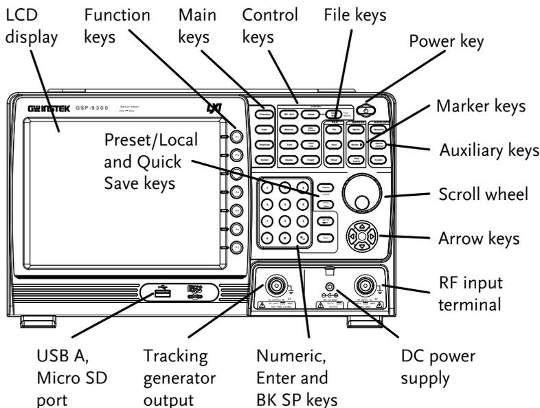
**LCD display**      800×600 color LCD display. The display shows the soft keys for the current function, frequency, amplitude and marker information.
