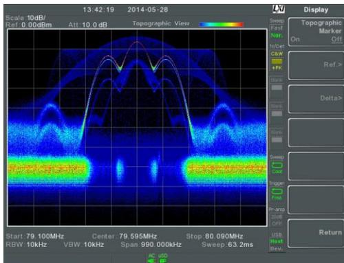
The topographic view shows the frequency of events. The topographic view is useful for observing smaller signals that have been overpowered by stronger signals or to easily observe intermittent events. Color is used to represent the frequency of an event. Red represents a high frequency of occurrence, while blue represents events that occur rarely.
