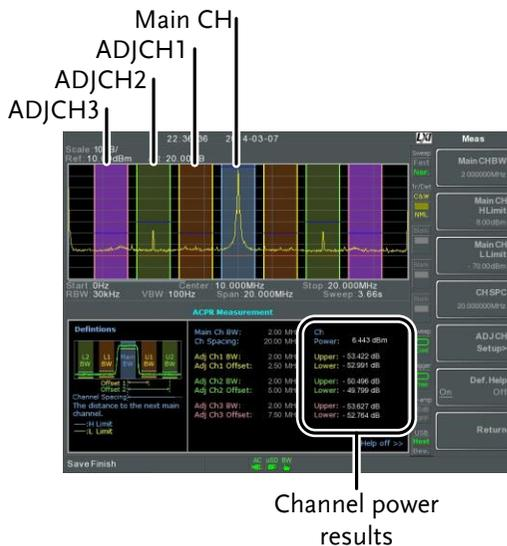
3. Press **Measure** > *Channel Analysis[F1]>ACPR Setup[F1]* > and set the following:
