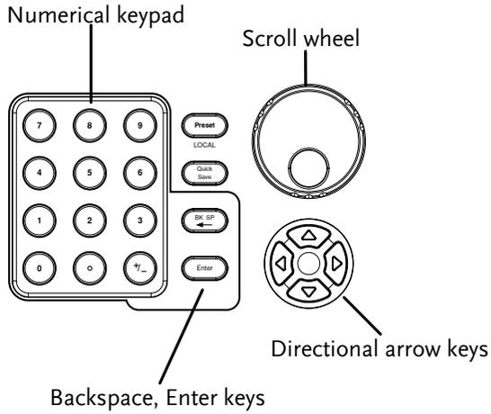
Parameter values can be entered using the numeric keypad, the scroll wheel and occasionally with the arrow keys.
