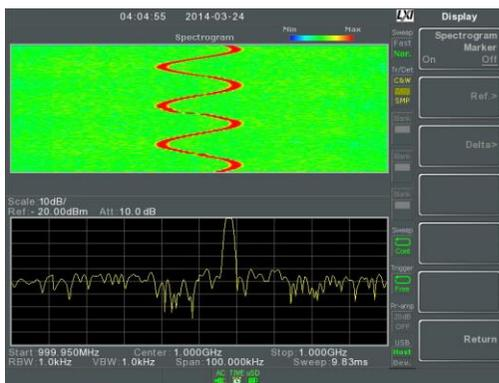
Displays both spectrographic and spectrum views of the signal.
