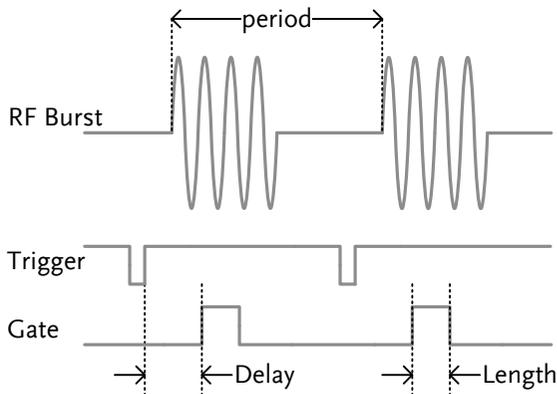
Example: The diagram above demonstrates the relationship between the input trigger, the input signal and the position of the gated sweep relative to the input signal.
