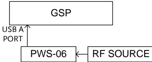
**Operation**                      1. Press
