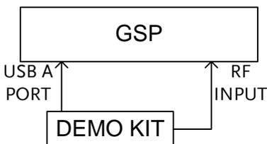
**Setup**                              1. Press Option Control > *Demo Kit*[F4]>*Demo Kit*[F1] and toggle the demo kit on.
