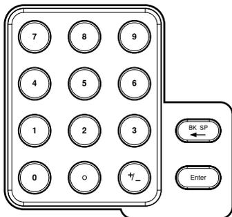
The numeric keypad is used to enter values and parameters. It is often used in conjunction with the arrow keys and scroll wheel.
