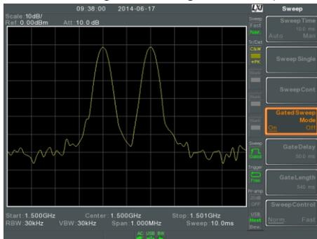
The example below shows the same signal with the gated sweep timed to sweep when only the desired frequency is output.
