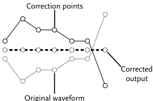
Example: The diagram above shows how amplitude correction is used to compensate for any losses or gains at specific frequencies.
