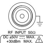
RF input port. Accepts RF inputs.
