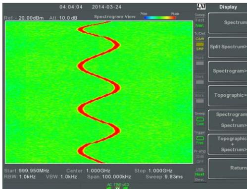
The Spectrogram view shows signals in both the frequency and time domain. The X-axis represents frequency, the Y-axis represents time and the color of each point represents the amplitude at a particular frequency & time (Red = high → dark blue = low).
