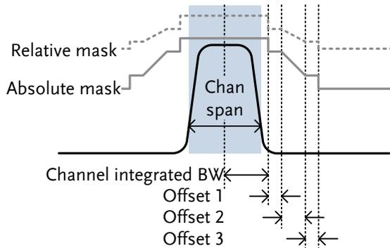
**Parameters** ChanIntegBW: Channel Integration Bandwidth. The ChanIntegBW is used to measure the in-channel
