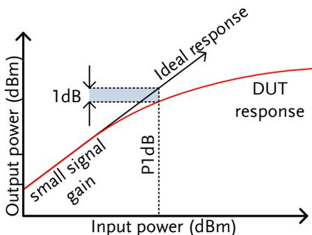
**P1dB Connection Setup** Connect the DUT to the RF input. Connect the tracking generator output to the DUT input. The DC output can be used to power the DUT if necessary.
