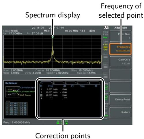
3. Press *Point Num*[F1] and choose a point number to edit. Point numbers can only be created in order. For example Point Num 2 can only be selected after Point Num 1 is created, and point Num 3 can only be selected after Point Num 2 is created and so on.
