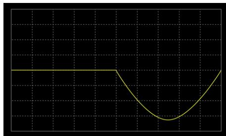
ARB 7 Sine wave, full-wave rectification(positive polarity)
