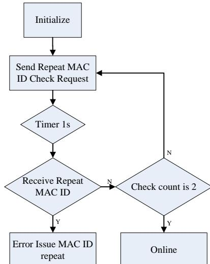
When each node connects to the network, it needs to send the MAC ID request check twice at an interval of 1 second and wait for 1 second after sending a request message. If the node does not receive a duplicate response message within the period, then go online successfully and become normal sending and receiving messages.
