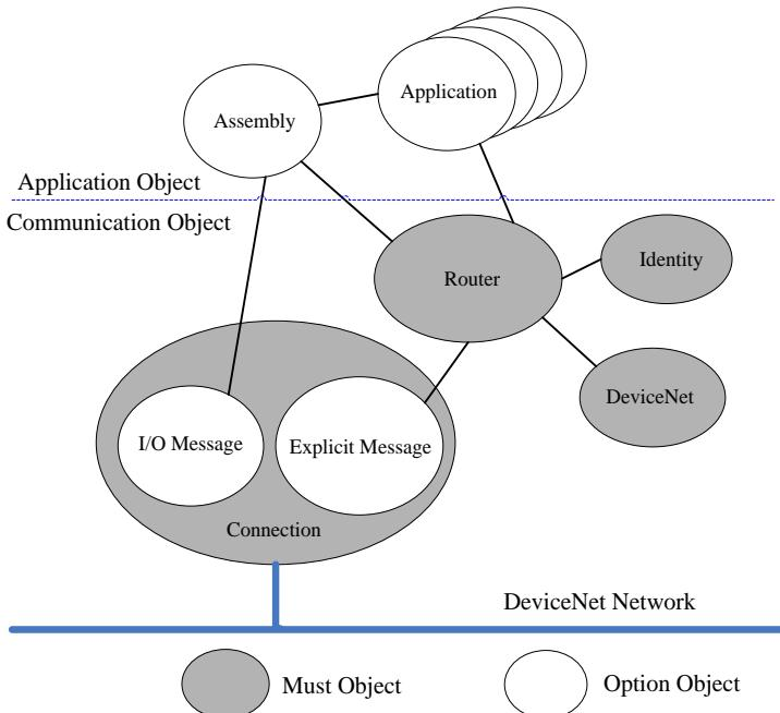
DeviceNet uses the object model to describe the network how to establish and manage device communication. Each device consists of communication object and application object. A DeviceNet can define the object and all of typical device objects contains Identity, Message Router, DeviceNet, Assembly, Connection and Application object. Device communication used Class, Instance, Attribute, Service to describe the structure encoding.
