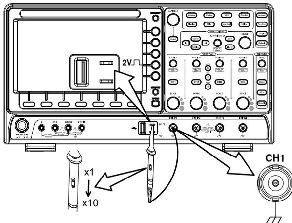
6. Capture Signal (Autoset) Press the *Autoset* key. A square waveform appears on the center of the screen. For Autoset details, see page 40.
