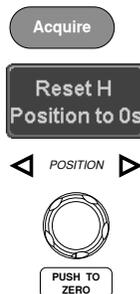
Alternatively, pushing the horizontal position knob will also reset the position to zero.
