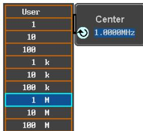
The variable knob can be used to select one. Press again on the *Center* button; the variable knob can now be used to set the frequency in increments of the chosen step resolution.
