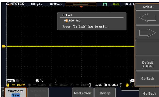
8. Use the Left and Right arrow keys to select a base unit and use the variable knob to increase the offset by that base unit, as shown in the Offset window.
