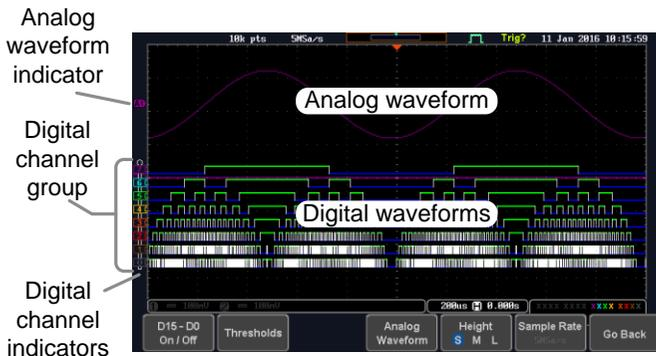
Analog Waveform Used to show the position of the analog waveform outputs.
