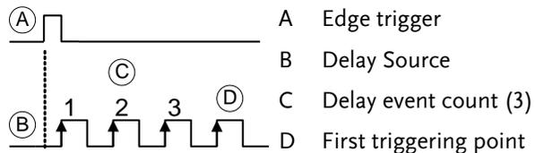
Delay trigger example (by time)
