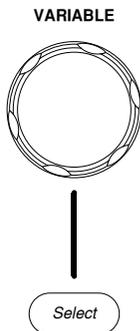
The Variable knob is used to increase/decrease values or to move between parameters.
