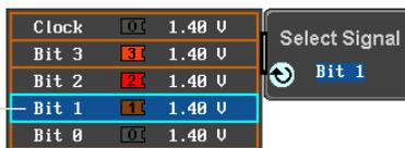
8. Next, press *Select Ch* and select which channel is assigned to the bit selected above.
