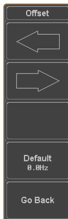
8. Default can be pressed to set the Offset to 0.0Hz.
