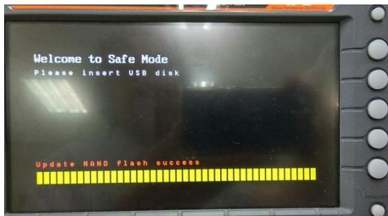
6. Restart the oscilloscope manually. Check the firmware version by pressing the “Utility” → “System” → “System Info”. The system information screen that it is being updated.
