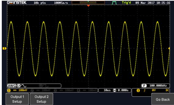
3. Select *Output setup 1* or *Output setup 2* button to set and turn on the power supply. For example, press the *Output setup 1* button. The following diagram will appear on the display.
