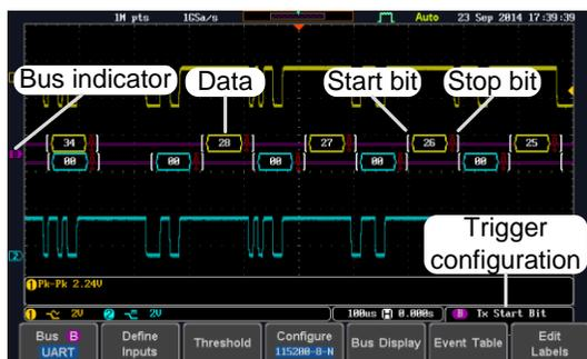
Start Bit/Start of Frame [ The Start bit is shown as an open bracket (Serial bus data only).
