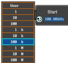
The variable knob can be used to select one. Press again on the *Start* or *Stop* button; the variable knob can now be used to set the frequency in increments of the chosen step resolution.
