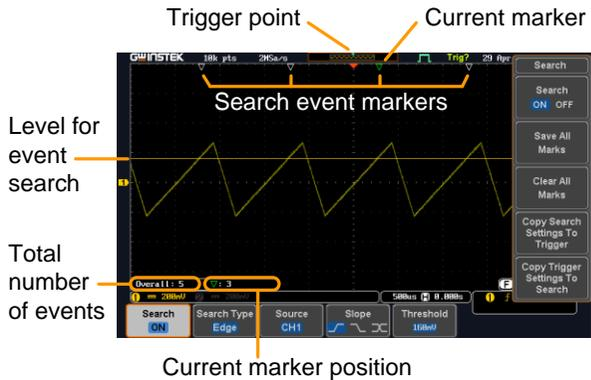
**Search Event Types** Edge, Pulse Width, Runt, Rise and Fall Time, FFT Peak\*, Logic and Bus
