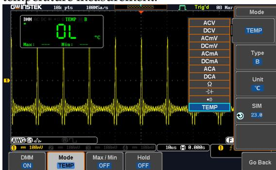
2. Select the thermocouple type. Thermocouple = B E, J, K, N, R, S, T
