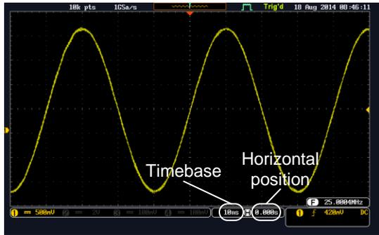
**Run Mode** In Run mode, the memory bar and waveform size keep their proportion. When the timebase becomes slower, roll mode is activated (if the trigger is set to Auto).
