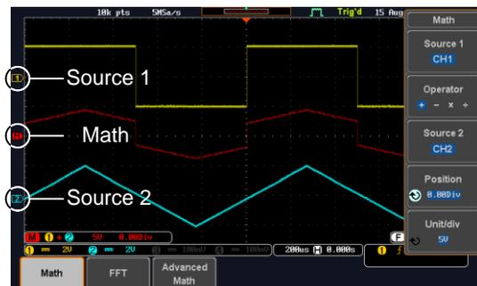
**Position and Unit** To move the math waveform vertically, press the *Position* key from the side menu and use the *Variable* knob to set the position.
