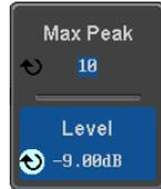
Select *Level* to set the threshold level for the search events. Any peaks above the threshold level will be seen as a search event.
