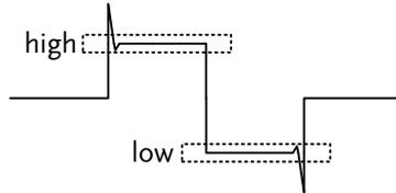
**Min-max** Sets the high-low values as the minimum or maximum measured values.
