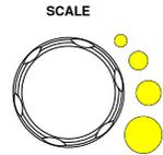
The vertical scale indicator on the bottom left of the display changes accordingly for the specific channel.
