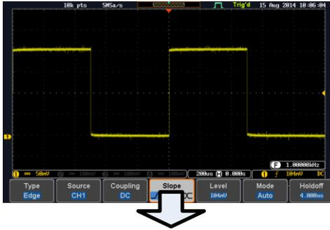
11. Press the relevant function key again to reduce the bottom menu. For example: press the Trigger Menu key to reduce the trigger menu.
