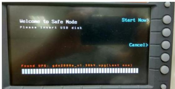
3. When the firmware file of USB flash disk has been recognized by oscilloscope, a message of “Found UPG: xxx.upg” will appear on the lower corner.
