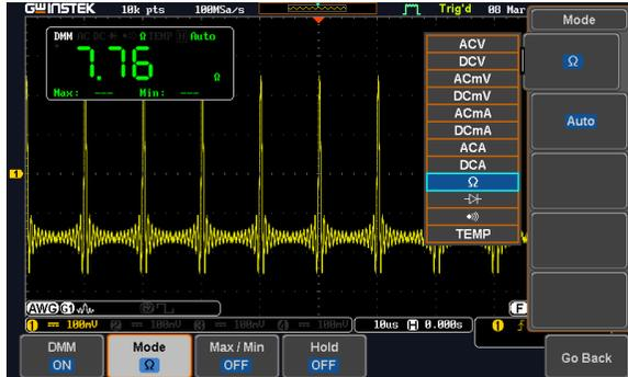
2. Use the *Variable* knob to select the required measurement and press the *Select* key to confirm.
