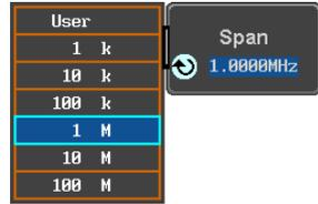
The variable knob can be used to select one. Press again on the *Span* button; the variable knob can now be used to set the frequency in increments of the chosen step resolution.
