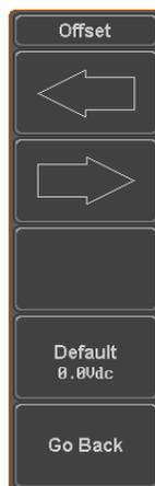
9. Default can be pressed to set the Offset to 0.00Vdc.
