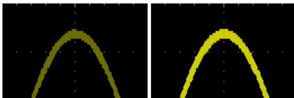
Graticule Intensity 4. To set the graticule intensity, press *Graticule Intensity* from the side menu and edit the intensity value.
