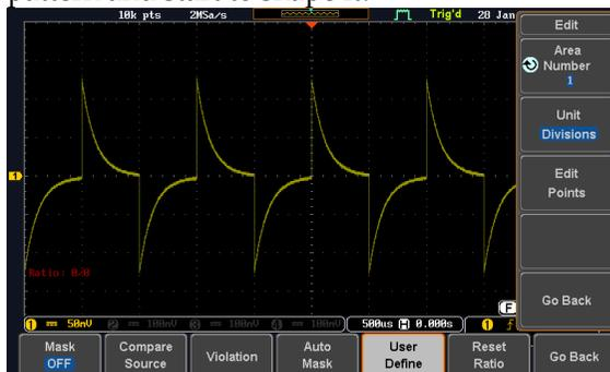
4. Press the *Unit* button from the side menu and use the *Variable* knob to either select *Divisions* (graticule division fractions) or *Current* (Actual oscilloscope X- and Y-axis scale units) as the points position units.
