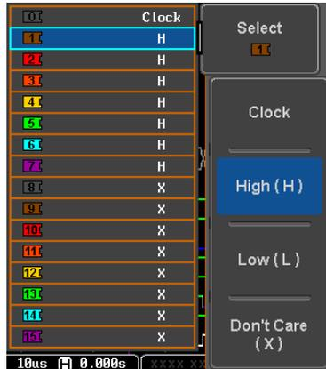
6. Next, select a logic level for the selected channel, or set the selected channel as the clock signal.
