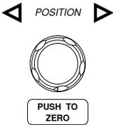
The Position knob is used to position the waveforms/traces horizontally on the display screen. Pressing the knob will reset the position to zero.
