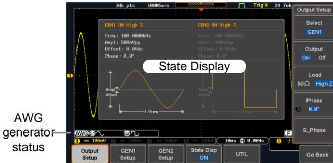
**State Display**      The state display is used to visually show the major channel settings when you are in the AWG menu.
