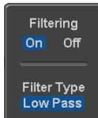
3. Press *Filter Type* and select low, high, or band pass filter.
