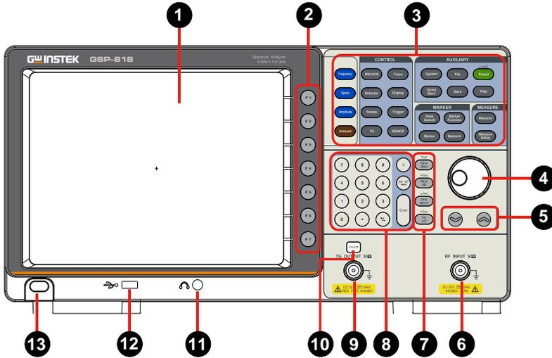
1. LCD 800x600 color LCD display. The display shows the soft keys for the current function, frequency, amplitude and marker information.
