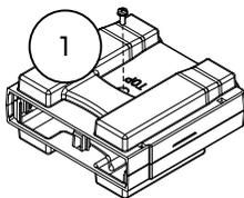
2. Line-up the bottom cover with the notches in the output terminals.
