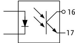
Photocoupler input: 30V max, 8mA, max.
