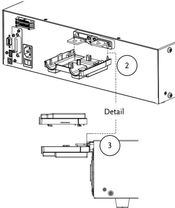
4. Use your thumb to slide the terminal covers shut, as shown in the diagram below.
