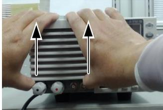
2. Remove the filter from the grill and replace with GW Instek part number: PEL-010.
