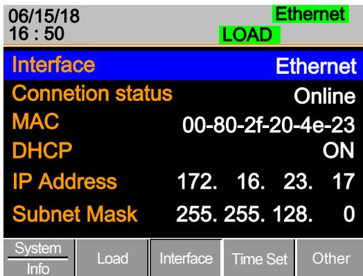
Use the Selector knob to edit DHCP, IP Address, Subnet Mask and Gateway setting.
