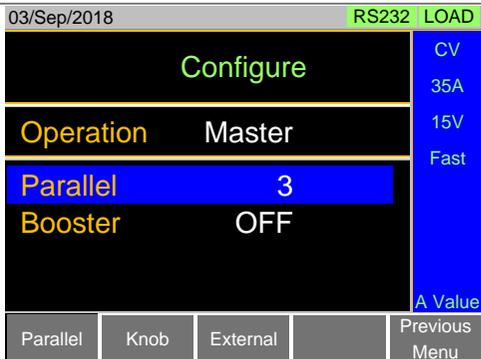
4. On the slave units, press **Main** > *Configure* [F5] > *Next Menu* [F4] > *Parallel*[F1] > and set *Operation* to *Slave*.
