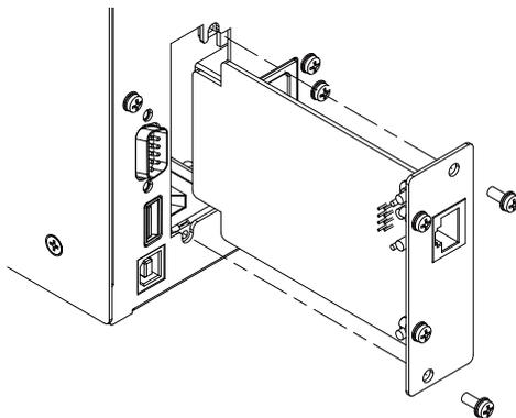
Use the screws that were removed from step 1 to secure the ethernet card.
