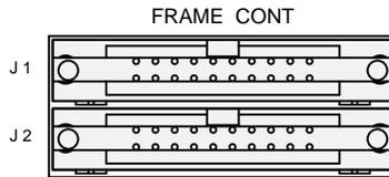
J1: The J1 connector is assigned to external control.
