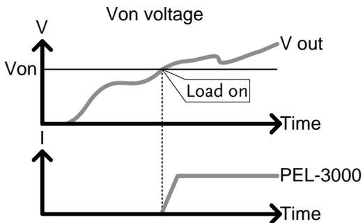
**Operation** Press **Main** > *Configure*[F5] > *Other*[F2] and set the *Von Voltage* level.
