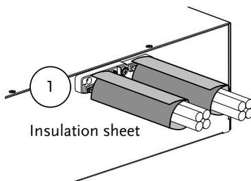
Secure the insulation sheets using the supplied velcro fasteners. 2 fasteners should be used for each sheet.
