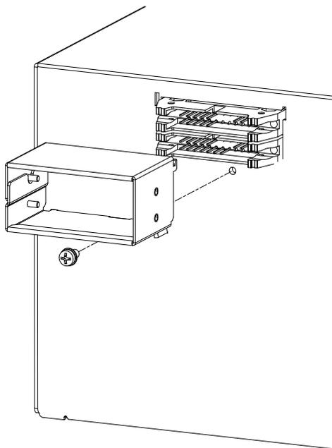
Install the terminal cover as shown in the picture below (for PEL-3000 series).
