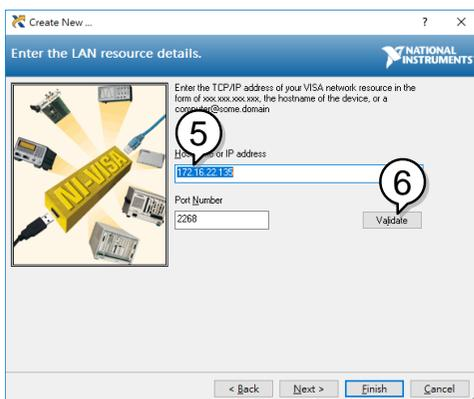
A popup will appear if a connection is successfully established. If not, check the Load device IP address configure. Then click OK button and Next button.
