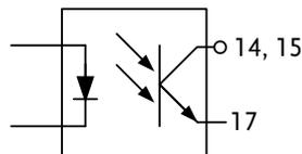
Photocoupler input: 30V max, 8mA, max.
