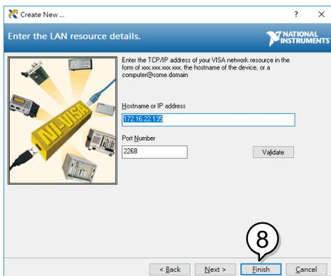
You can see the network device is setup successful. Click *Open VISA Test Panel*.
