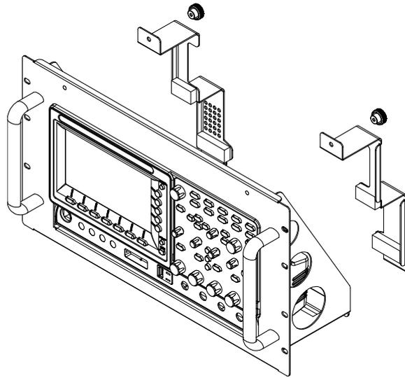
2. Insert the left and right fasteners into the two holes in the bottom cover.
