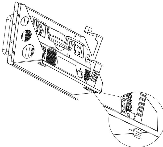
3. Screw the left and right fasteners to the rack with the embossed nuts(6010-L00040S1).
