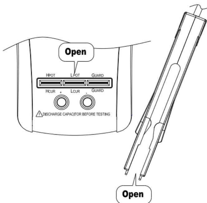
When “OPE n” appears on the sub display, make the terminal or the SMD test probe open, and press the CAL button to start the open calibration. About 30 seconds later, the result of the open calibration appears on the main display. If the result is “pass”, press the CAL button to proceed to the next step. If the result is “fail”, press the CAL button to exit the function.
