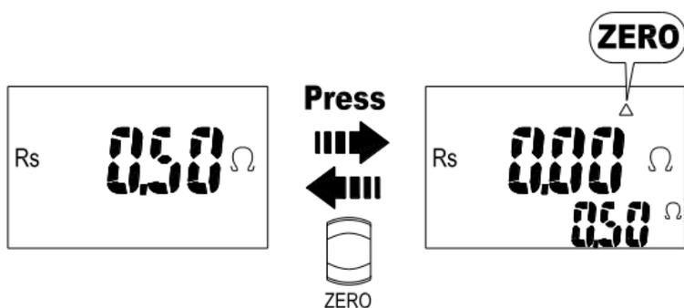
The Zero mode records the current input value as a reference and displays the reference on the sub display. Any inputs after this will be subtracted from the reference value and displayed on the main display. To use the Zero mode, follow the steps below.
