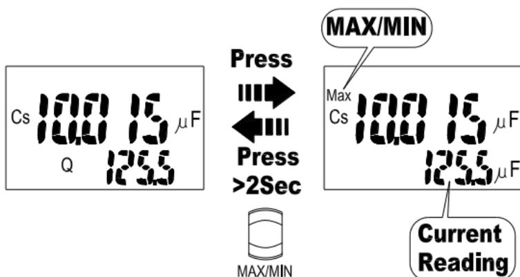
The MAX/MIN mode records the maximum and the minimum input values. When the inputs go below the recorded minimum value or above the recorded maximum value, the meter beeps and records the new value.
