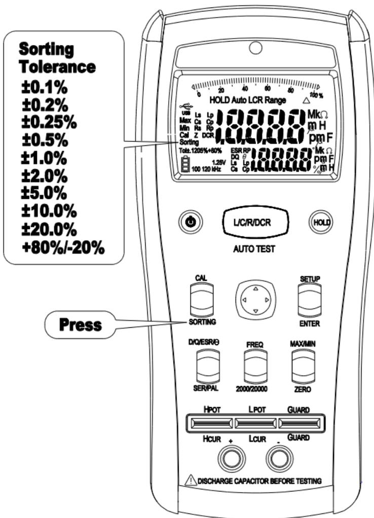
To check the accuracy of a part, press the SORTING button to enter the sorting mode. The sorting result appears on the main display, and the current value appears on the sub display.
