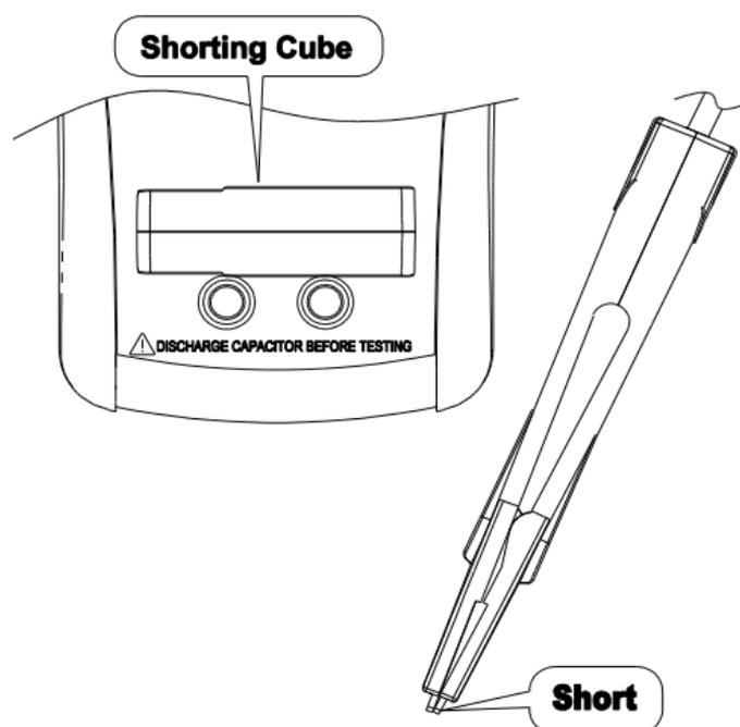
When “Srt” appears on the sub display, short the terminals or the SMD test probe, and then press the CAL button to start the short calibration. About 30 seconds later, the result of the short calibration appears on the main display. If the result is “pass”, press the CAL button to complete the calibration. If the result is “fail”, press the CAL button to exit the function.
