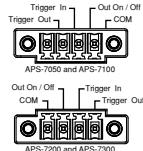
Connector for controlling the TRIGGER IN, TRIGGER OUT and OUT ON/OFF states.
