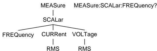
**Command types** There are a number of different instrument commands and queries. A command sends instructions or data to the unit and a query receives data or status information from the unit.
