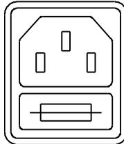
The power socket accepts AC mains voltage, 115V or 230V.
