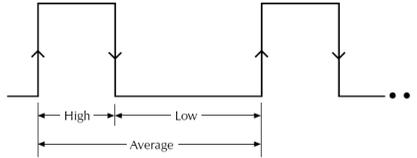
The high and average measurements are triggered by the rising edge of the pulse current are performed for the time specified for the measurement.
