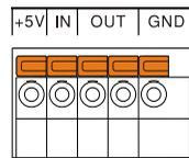
**Wiring Method** A thin screwdriver or similar tool will need to be inserted into the release mechanism (highlighted in orange in the figure above) to open the terminals. Insert an exposed wire into the terminal and release the mechanism to lock the wire into place.
