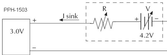
Conditions            To protect the high-speed power supply when operating as a current sink, the following two conditions must be met:
