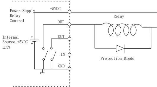
**Warning:** Do not short the 5VDC terminal to the chassis, earth or to the control port GND, otherwise it may damage the unit.
