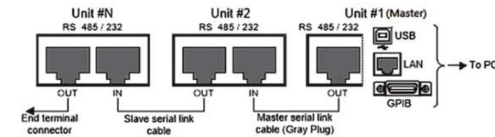
Provide RS-232, RS-485, USB, GPIB and LAN for PC to remote control Master PSU-Series. RJ-45 connector on the rear panel can connect up to 31 units.
