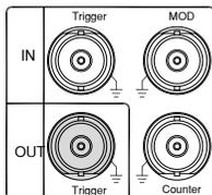
Marker output signal. Used for Sweep, Burst and ARB mode only.
