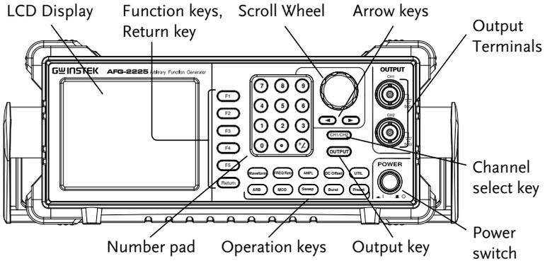
LCD Display TFT color display, 320 x 240 resolution.
