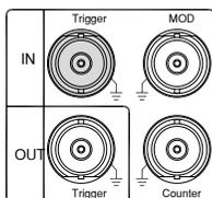
External trigger input. Used to receive external trigger signals.
