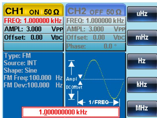
3. Use the arrow keys and scroll wheel or number pad to enter the carrier frequency.
