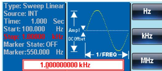
4. Use the arrow keys and scroll wheel or number pad to enter the Stop/Start frequency.
