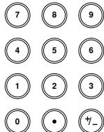
The digital keypad is used to enter values and parameters. The keypad is often used in conjunction with the arrow keys and variable knob.
