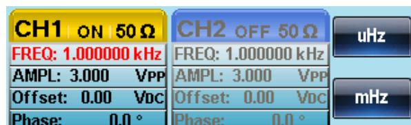
3. Use the arrow keys and scroll wheel or number pad to enter the frequency.
