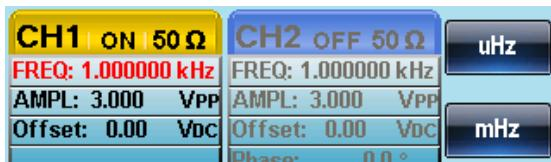
3. Use the arrow keys and scroll wheel or number pad to enter the carrier frequency.
