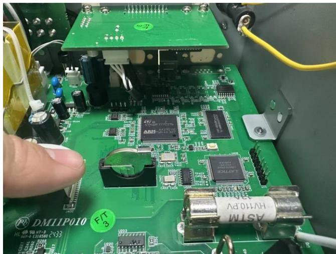
4. Gently remove the metal guard plate on top of the battery followed by pinching the battery out off the compartment with 2 fingers..
