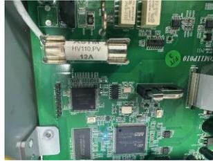
4. Pull the fuse out from the fuse holder with a flat-blade screwdriver. Be cautious Not to damage the printed circuit board (PCB).
