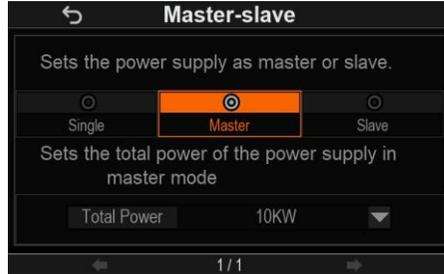
Master: The user can set the total power of up to 150 kW.
