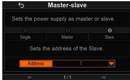
Slave: The user can set Slave units numbered from 1 to 10.
