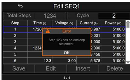
11. In the “Edit SEQ1” menu, rotate the Voltage Knob to “Edit” and press the Voltage Knob. This will enter the “Edit SEQ1 / Step1” first page setting menu.
