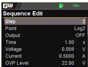
7. Scroll knob key to move to the Step field followed by clicking knob key to enter the field. Scroll knob key to select a step along with arrow keys to change among digits followed by clicking knob key to confirm the step to edit.
