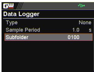
4. Scroll the knob key to move to the Type field. Click knob key followed by scrolling it to select a type for data log saving. Click knob key to confirm setting.
