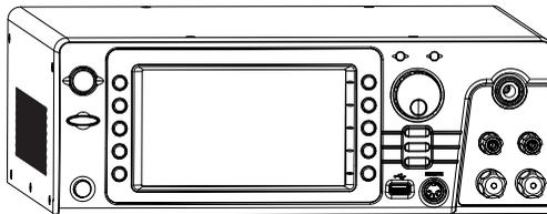
Tilt stand position Gently pull the 2 stands out from the bottom and the unit will be placed in the tilt stand position.
