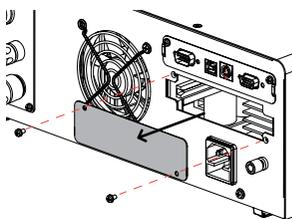
2. Insert the GPIB/LAN card into the opening of rear panel. Push the card gently until it is fully inserted followed by fastening the screws.
