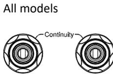
The OUTPUT terminal (red) and RETURN terminal (black) are used for CONT (Continuity) test.
