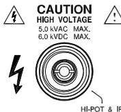
The HIGH VOLTAGE terminal output is used for outputting the testing voltage in ACW, DCW and IR tests. The terminal is recessed for safety. This terminal is used in conjunction with the RETURN terminal.
