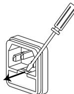
4. Replace the fuse in the fuse holder.
