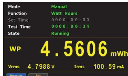
GPM-8310 provides a variety of measurement items and functions, including voltage, current, frequency, effective power, apparent power, reactive power, power factor, crest factor, total harmonic distortion, and can also measure the maximum current ratio. GPM-8310 is also equipped with the measurement function of power or current time integration for the DUT. Users set a period of time to perform instantaneous power
