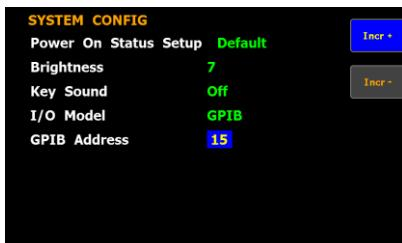
Option The range of GPIB Address is from **1 to 30**.
