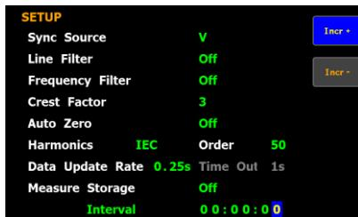
**Option** The setting range for Interval is from 00:00:00 to 99:59:59.
