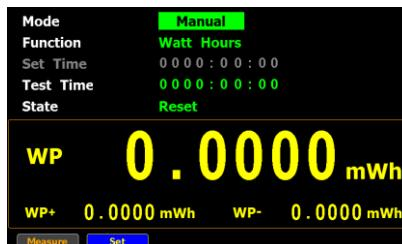
5. Press **Enter** button to enter **Mode** field. Use up and down arrow keys to toggle between Manual, Standard and Continuous mode. Press **Enter** button again to confirm your selection.
