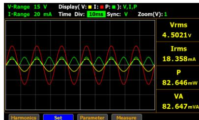
7. Press **Enter** button to enter Time Div field. Use up and down arrow keys to toggle between options. Press **Enter** button again to confirm your selection.
