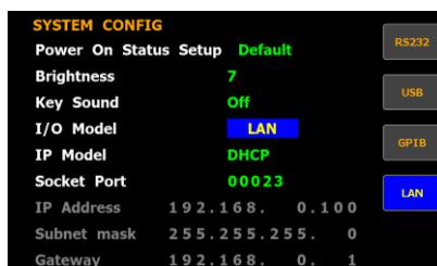
4. Press down arrow key to move cursor to **IP Model** field.
