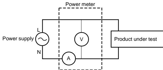
$$\text{Power loss} = (\text{Input voltage[V]})^2 / 2M\Omega$$
