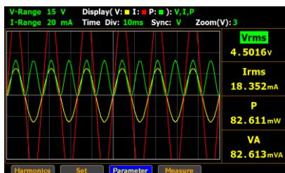
5. Press **Enter** button to enter the 1st parameter. Use up and down arrow keys to toggle between options. Press **Enter** button again to confirm your selection.
