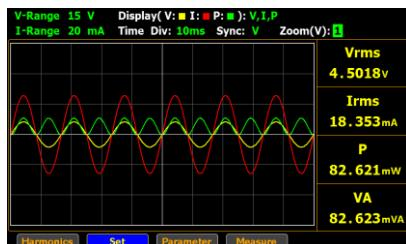
11. Press **Enter** button to enter **Zoom (V)** field. Use up and down arrow keys to toggle between options. Press **Enter** button again to confirm your selection.
