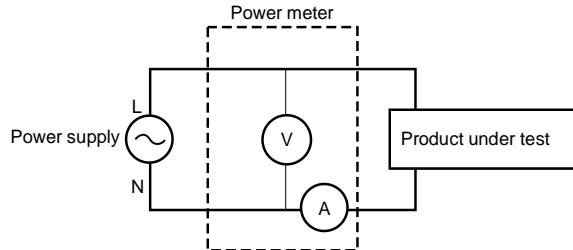
$$\text{Power loss} = (\text{Input current}[A])^2 \times 505\text{m}\Omega$$
