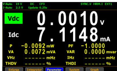
3. Press up, down, left and right arrow keys to select other desired measurement parameter.
