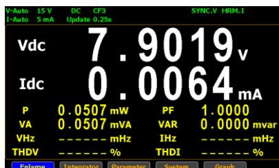
2. Press **Enter** button to switch display to simple mode.
