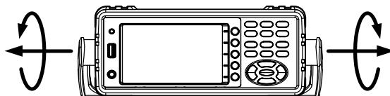
Pull out the handle sideways and rotate it clockwise for the several applications listed below.
