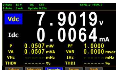
4. Press **Enter** button followed by using up and down arrow keys to switch display options for the selected measurement parameter.
