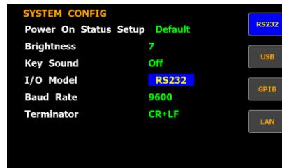
4. Press down arrow key to move cursor to **Baud Rate** field.
