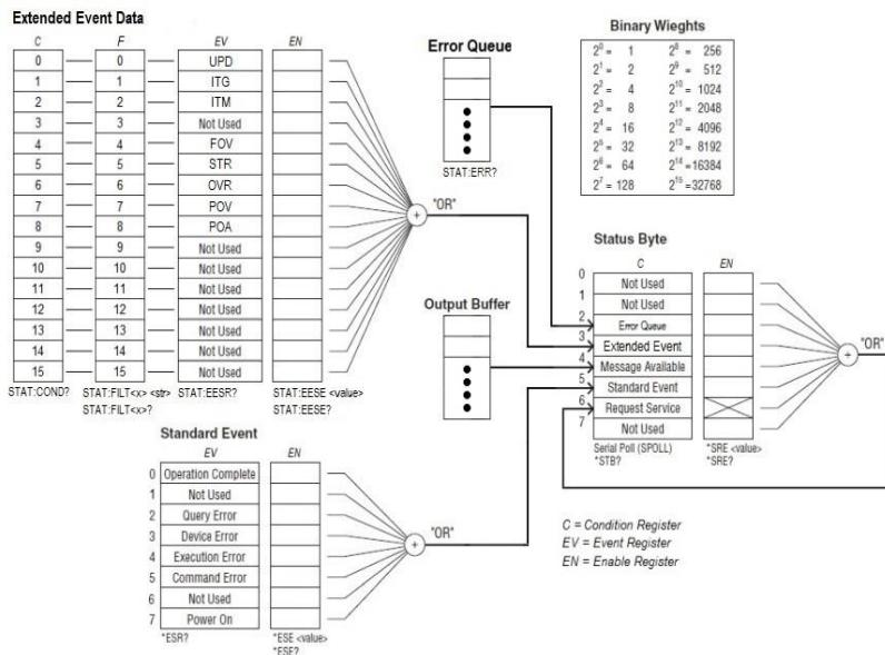
The extended event register receives information about changes in the condition register, which indicates the instrument's internal condition. The information is the result of edge detection performed by the transition filter.
