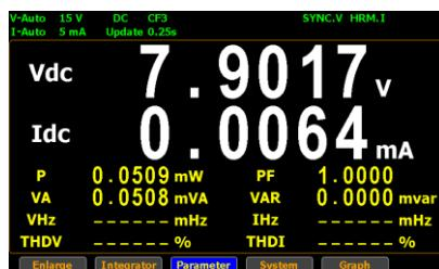
2. Press **Enter** button. The 1st measurement parameter will be highlighted in green.
