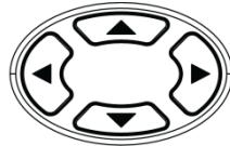
This four arrow keys are used to edit the parameters, browse the menu system and select the parameter range.
