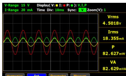
9. Press **Enter** button to enter **Sync** field. Use up and down arrow keys to toggle between options. Press **Enter** button again to confirm your selection.
