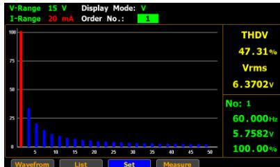
8. Press **Enter** button to enter Order No. field. Use up and down arrow keys to toggle between options. Press Enter button again to confirm your selection.
