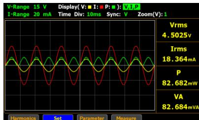
5. Press **Enter** button to enter **Display** field. Use up and down arrow keys to toggle between options. Press **Enter** button again to confirm your selection.
