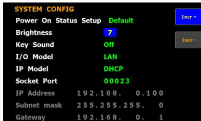
Option 1 - 10 The display is the darkest when set to 1. On the contrary, it turns out the brightest when set to 10.
