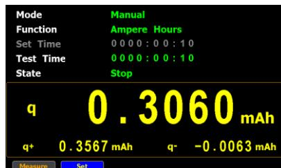
3. Press the **Reset** button in the front panel to clear integrator.
