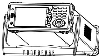
Rotate the handle for tilt stand.
