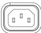
Power cord socket accepts AC mains, 100 ~ 240V, 50/60Hz.
