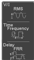
V/I (Voltage/Current) Pk-Pk, Max, Min, Amplitude, High, Low, Mean, Cycle Mean, RMS, Cycle RMS, Area, Cycle Area, ROVShoot, FOVShoot, RPRESshoot, FPRESshoot
