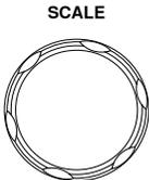
The Scale knob is used to change the horizontal scale (TIME/DIV).
