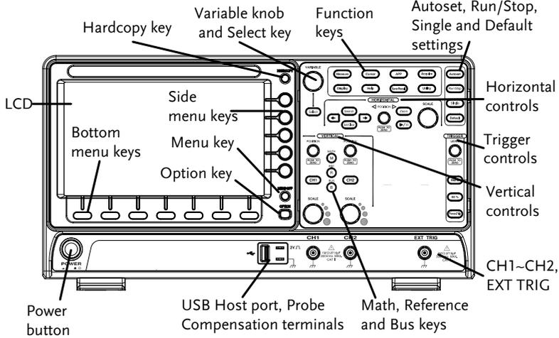
**LCD Display**      8" WVGA TFT color LCD. 800 x 480 resolution, wide angle view display.
