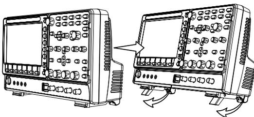
**Stand** To stand the scope upright, push the legs back under the casing as shown below.
