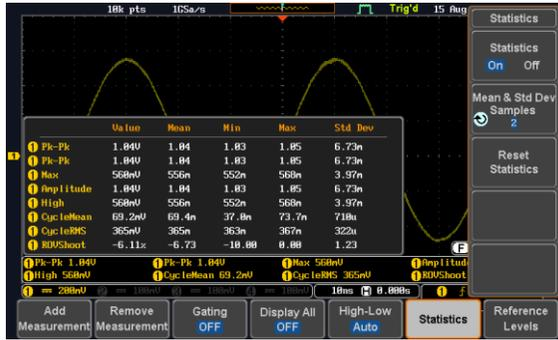
**Reset Statistics** To reset the standard deviation calculations, press *Reset Statistics*.
