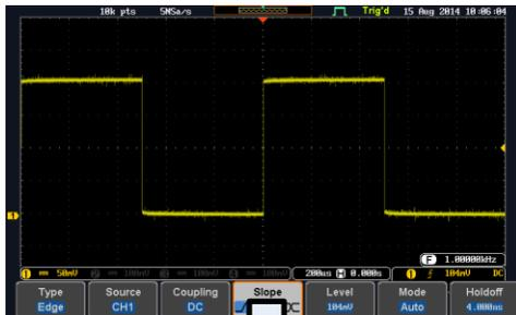
11. Press the relevant function key again to reduce the bottom menu. For example: press the Trigger Menu key to reduce the trigger menu.
