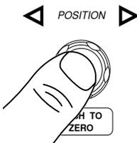
Alternatively, pressing the *Acquire* key and then pressing *Reset H Position to 0s* from the bottom menu will also reset the horizontal position.
