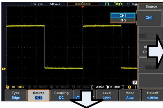
12. Press the *Menu Off* key to reduce the side menu, press again to reduce the bottom menu.
