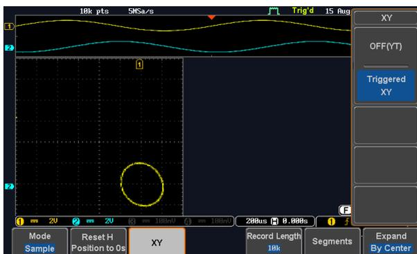
To move the XY waveform position, use the vertical position knob: Channel 1 knob moves the XY waveform horizontally and Channel 2 knob moves the XY waveform vertically.
