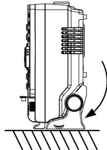
**Leaning Position**                Pull the feet back to have the instrument leaning back.
