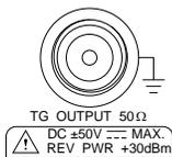
The Tracking Generator (TG) output source.
