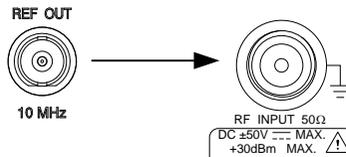
3. Press **Frequency** > *Center[F1]* and enter 10MHz. This is the output frequency of the REF out signal.
