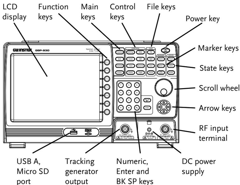
**LCD Display**      800×600 color LCD display. The display shows the soft keys for the current function, frequency, amplitude and marker information.
