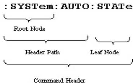
**Figure 5 Command Header**
