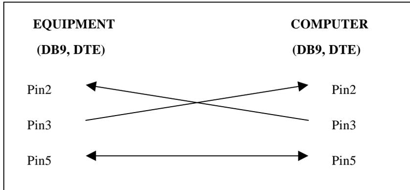
Figure 2 Wiring configuration for DB9 to DB9
