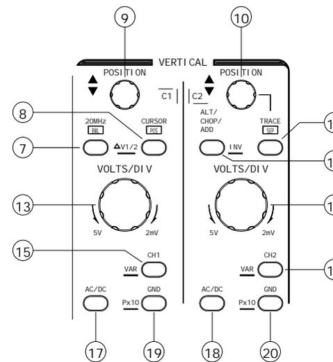
**(7).20MHz BWL** – Pushbutton with indicator LED.
