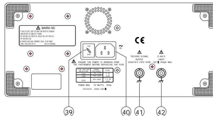
(39)**Line voltage selector and input fuse holder**—Select power source and contain the primary power fuse
