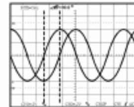
**NOTE. When the VOLTS/DIV or the TIME/DIV controls are in uncalibrated setting, the V and T measurement values will be displayed with divisions.**
