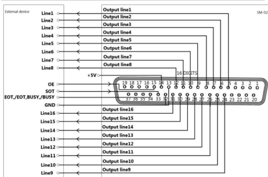
**Pattern value formats** The 16bit SM-02 DIGITAL I/O ADAPTER can output binary bit patterns from 0 to 1111111111111111. Before this, a decimal pattern value (0-65535) should be set from the front panel. For example, if you want output lines 8 and 2 to be high (0000000010000010), you should set the pattern value as 130.
