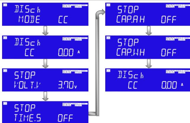
Setting battery discharge CC mode, DISCH CC, LCD show "DISCh", middle 5 digit LCD display "CC", setting range 0.00A to full scale.
