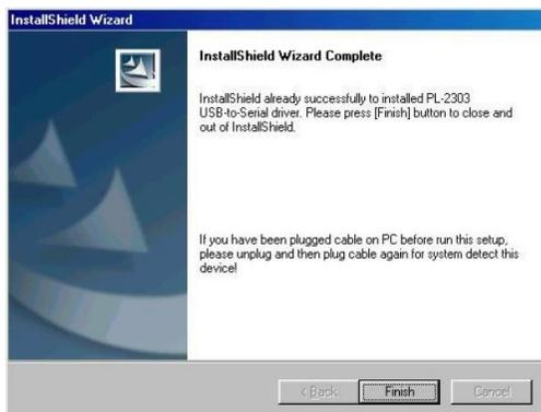
2. After the installation, connect the PEL-5000C series and PC with USB. Then select the item USB to Serial Port (COM3), set the BAUD-RATE and Flow control to 115200bps and Hardware to control PEL-5000C series with COM3.
