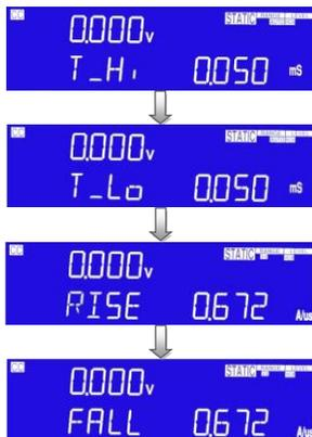
Press DYN setting key, LED will ON setting level High Period, Middle 5 digit LCD display will show "T-Hi" Right 5 digit LCD display will show setting value, the unit is "ms", the T-Hi set range from 0.010 ms to 9999 ms step 0.001ms by rotating the setting knob.
