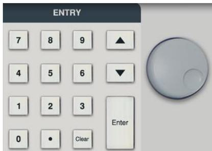
**Rotary Knob** The ROTARY knob and ARROW keys are used to increase or decrease the set values.
