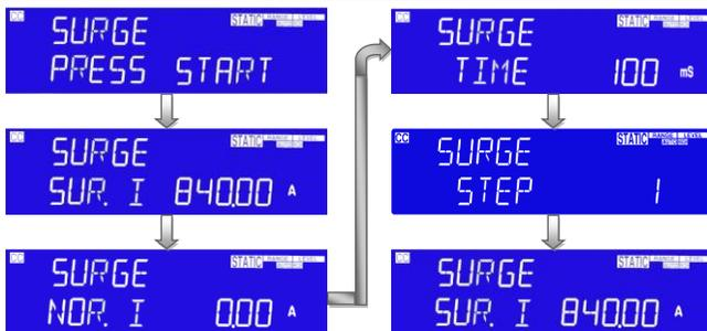
Set SURGE testing surge current, unit is A, setting range 0.00A to full scale.
