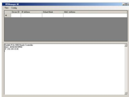
2. It will be shown the installation which has been searched on the screen, click it and select the Set IP Address bellows Config:
