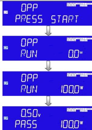
8. The UUT's output voltage drop-out lower than the threshold voltage (V-th setting), and the OPP trip point is between W\_Hi and W\_Lo limitation, then Right 5 digits LCD display will shows "PASS", otherwise shows "FAIL".
