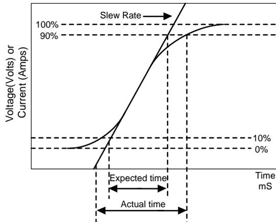
Therefore, both minimum transition time and slew rate must be considered when determining the actual transition time. Following detail description is excluding in specification sheet.
