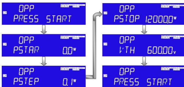
PSTAR: setting the start power, the LCD display shows “OPP” on left 5 digit LCD display, middle 5 digit LCD display “PSTAR”, right 5 digit LCD display setting value, the unit is “W”, the setting range is 0.00W to the full scale of the CP mode specification. The setting is by rotating the setting knob.
