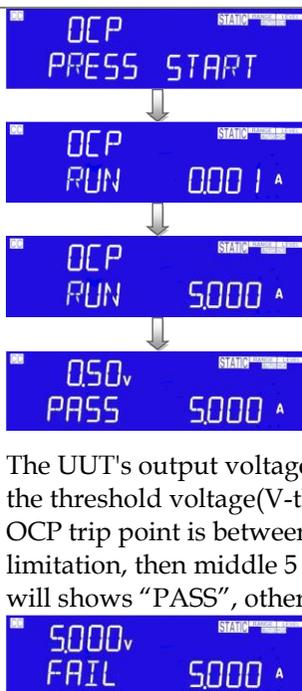
8. The UUT's output voltage drop-out lower than the threshold voltage(V-th setting), and the OCP trip point is between I\_Hi and I\_Lo limitation, then middle 5 digits LCD display will shows "PASS", otherwise shows "FAIL".
