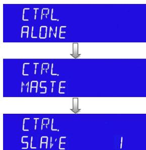
The following procedure should be followed before applying power on Master/Slave mains:
