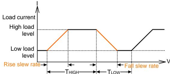
The dynamic waveform can also be set up via the optional computer interface. Dynamic waveform settings made from the front panel of the load module can also be saved in the memory of the PEL-5000C series Electronic Load. For the store/recall procedure and the computer command set please refer to the relevant operating manual for the PEL-5000C series Electronic Load.
