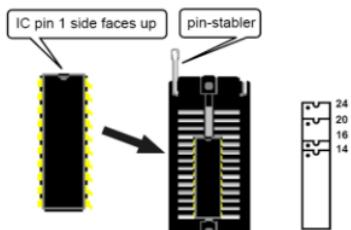
**STEP2.** Use **TYPE** to switch "TTL 74", "CMOS40", "CMOS45", "DRIVER" families.
