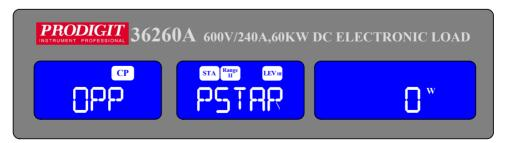
5.14.1.5. Press up key, set step load watt 5W, press OPP key to the next step.
