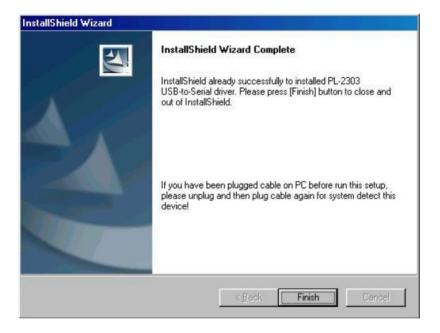
2.After the installation, connect the 36000A series and PC with USB. Then select the item USB to Serial Port (COM3), set the BAUD-RATE and Flow control to 115200bps and Hardware to control 36000A series with COM3.
