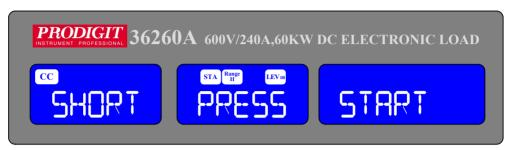
5.15.1.2. Press UP key, setting Short time to 10000ms, press Short key to The next Step.
