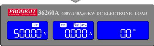
PSTAR: setting the start power, The LCD display shows "OPP" on Left 5 digit LCD display, Middle 5 digit LCD display"PSTAR", Right 5 digit LCD display Setting value, the unit is "W", the setting range is 0.00W to the full scale of The CP mode specification. The setting is by rotating the setting knob.
