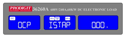
5.13.1.5. Setting step load current 0.01A, press OCP key to the next step.
