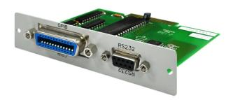
Fig 2-2 36000A Series GPIB & RS232 interface
