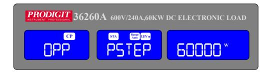
PSTOP: setting the stop power, The LCD display shows "OPP" on Left 5 digit LCD display, Middle 5 digit LCD display "PSTOP", Right 5 digit LCD display setting value, the unit is "W", the setting range is 0.00W to the full scale of the CP mode specification. The setting is by rotating the setting knob.
