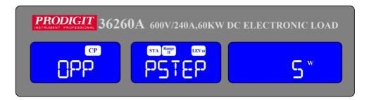
5.14.1.6. Press up key, set stop load watt 100W, press OPP key to the next step.
