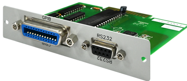
Fig 2-2 36000E Series GPIB & RS232 interface
