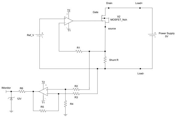
Fig 3-3 An equivalent circuit in terms of the current monitor
