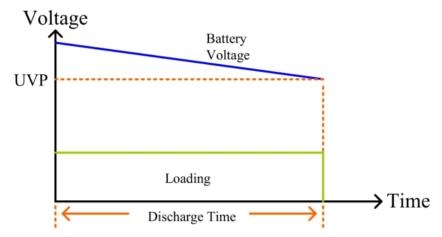
Fig 5-16 TYPE 1 Battery Discharge Figure
