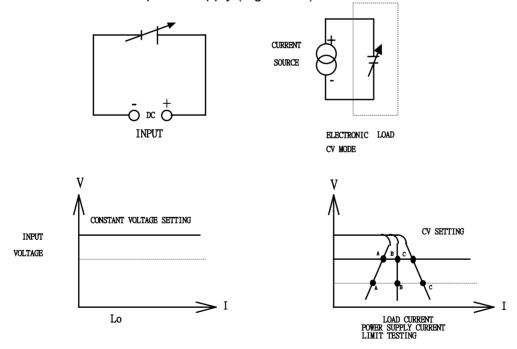
Fig 5-5 Constant Voltage mode application
