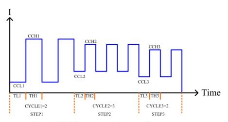
Fig 5-18 TYPE 4 Battery Discharge Figure
