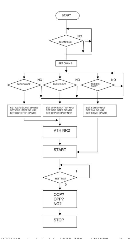
Fig 5-13 34000E series electronic load OCP, OPP, and SHORT operation flow chart
