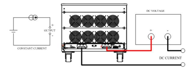
Fig 5-10 constant current source connection
