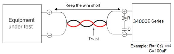
Fig 2-10 Length of wiring
