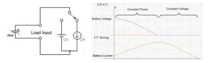
Fig 5-9 Application of CP to CV operation mode
