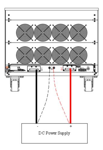
Fig 5-2 Remote voltage sense connections
