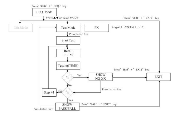
Fig 3-8 TEST MODE OPERATION FLOW-CHA
