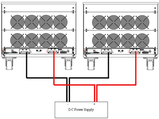
Fig 5-12 34000E series load parallel operation
