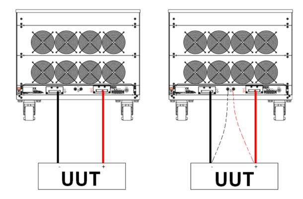
Fig 3-2 typical connection of 34000E series load module
