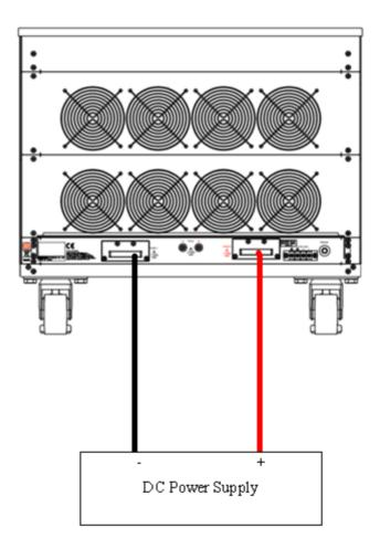
Fig 5-1 Local voltage sense connections
