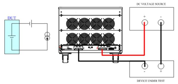
Fig 5-11 Zero-Volt loading connection
