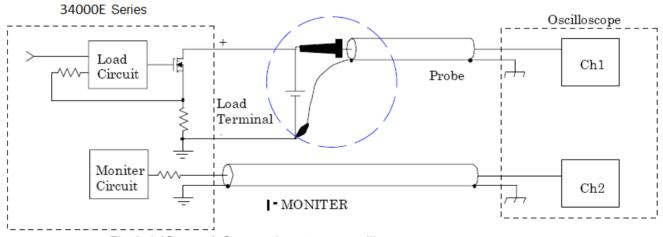
Fig 3-4 (Correct) Connections to an oscilloscope
