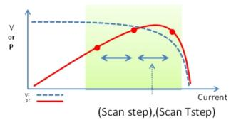
Enter Scan step (current step width) and Scan Tstep (step time) when searching max power)
