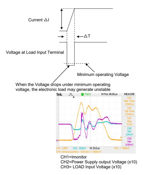
Fig 2-9 Waveform example: Generate unstable oscillation
