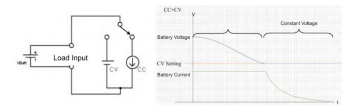
Fig 5-8 CC+CV mode operation application
