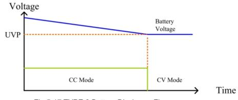
Fig 5-17 TYPE 2 Battery Discharge Figure
