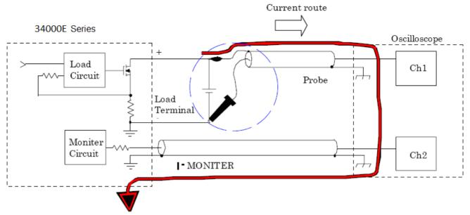
Fig 3-5 (Wrong) Connections to an oscilloscope
