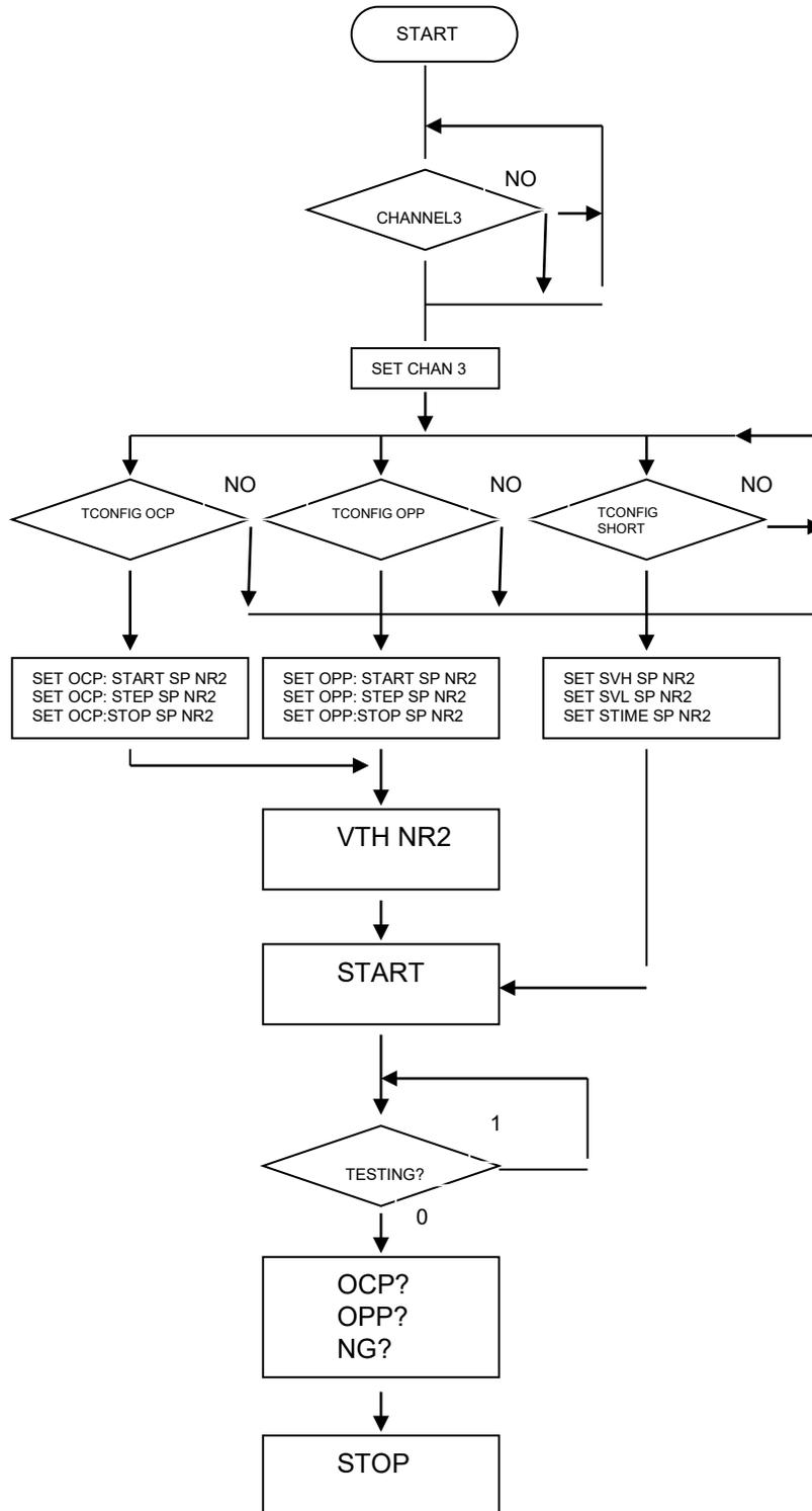
Fig 5-13 34000A series electronic load OCP, OPP, and SHORT operation flow chart
