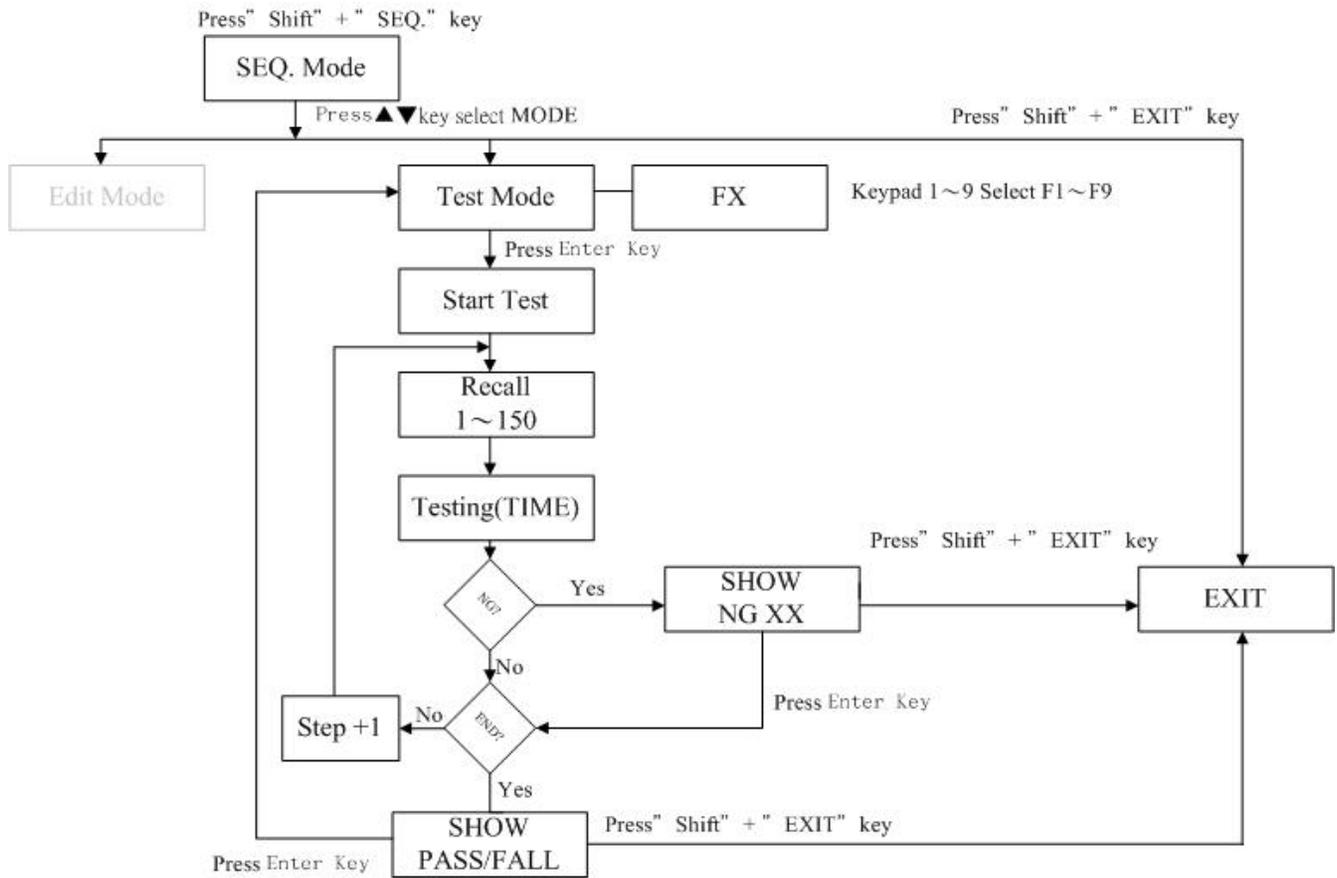
Fig 3-8 TEST MODE OPERATION FLOW-CHA
