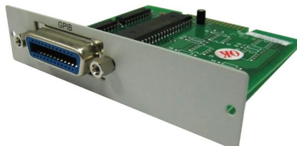
Fig 2-4 34000A Series GPIB interface
