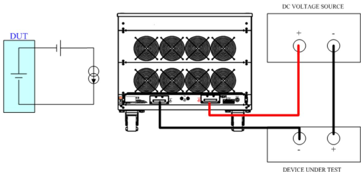
Fig 5-11 Zero-Volt loading connection
