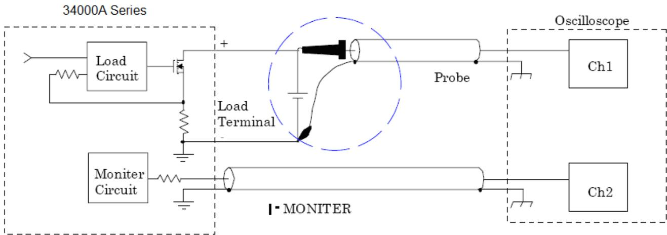
Fig 3-4 (Correct) Connections to an oscilloscope
