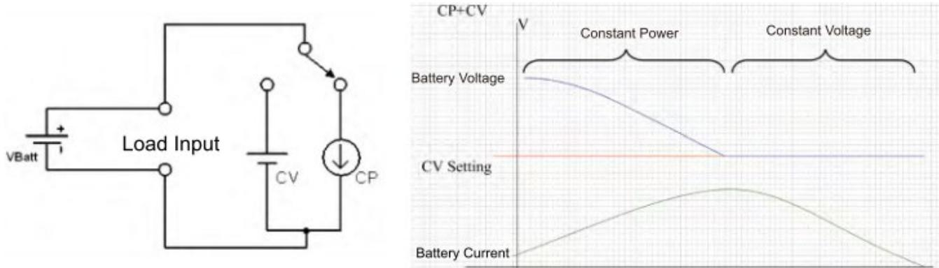
Fig 5-9 Application of CP to CV operation mode
