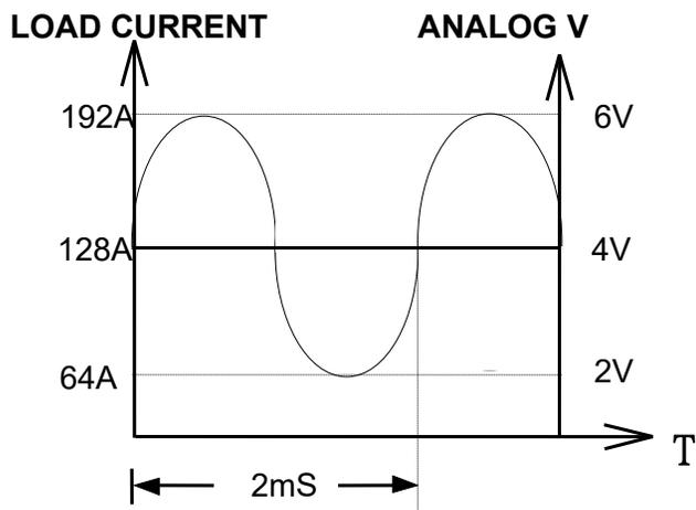
Fig 3-6 Analog programming example
