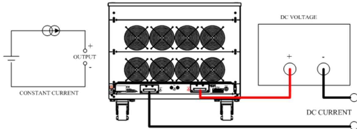
Fig 5-10 constant current source connection
