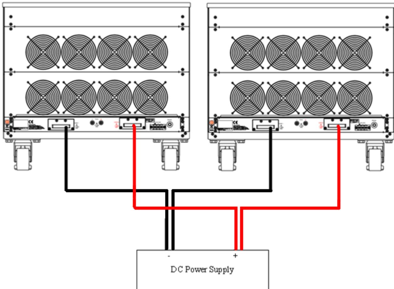
Fig 5-12 34000A series load parallel operation
