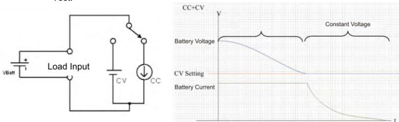
Fig 5-8 CV + Current Limit mode operation application
