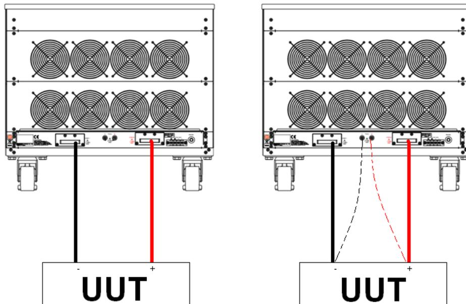
Fig 3-2 typical connection of 34000A series load module
