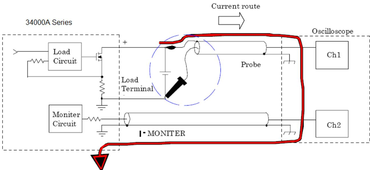
Fig 3-5 (Wrong) Connections to an oscilloscope
