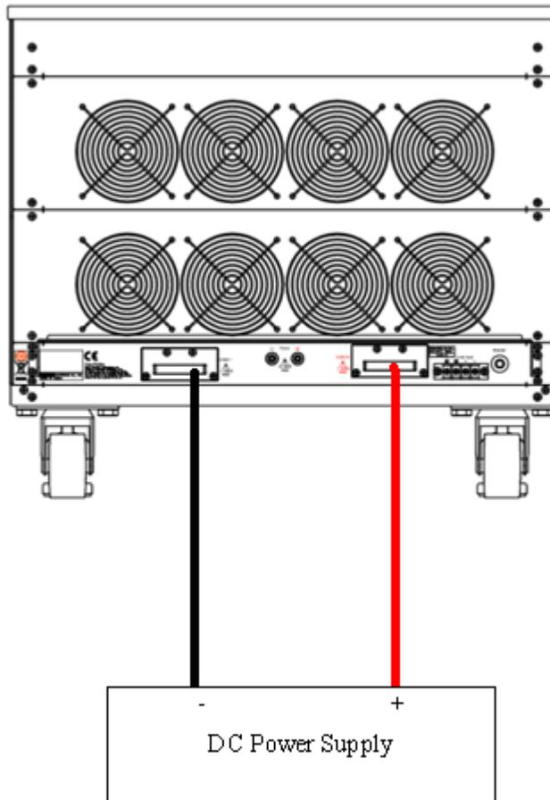
Fig 5-1 Local voltage sense connections
