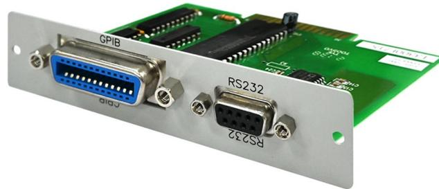
Fig 2-2 34000A Series GPIB & RS232 interface
