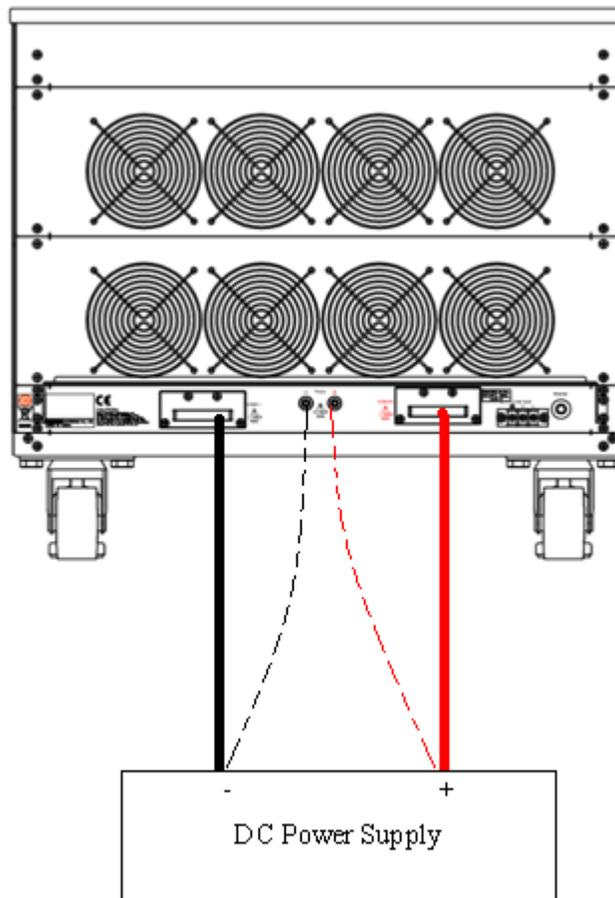
Fig 5-2 Remote voltage sense connections
