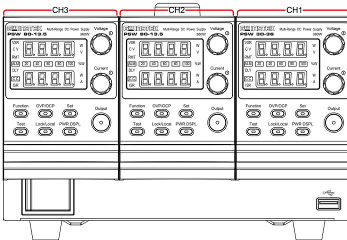
1 Voltage Knob      Voltage
