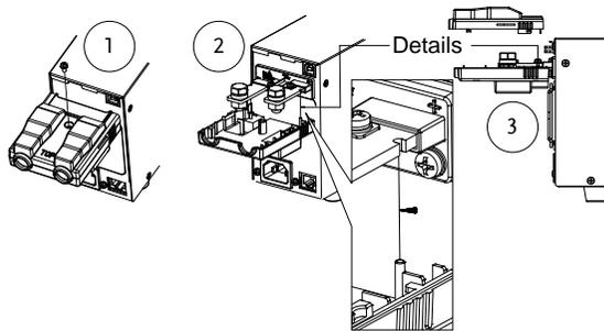
4. Use your thumb to slide the terminal covers shut, as shown in the diagram below.
