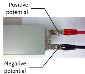
Connection with voltage sense wiring
