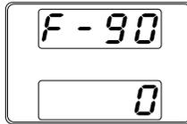
3. Rotate the voltage knob to change the F setting on each channel.
