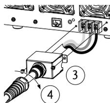
4. Screw the power cord sheath back onto the cover.
