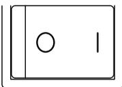
Used to turn the power on/off (with trip function).
