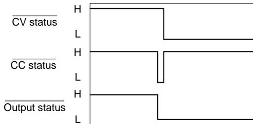
**CV MODE:** The diagram below shows the output status lines
