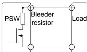
Bleeder resistor is designed to dissipate the power from the power supply filter capacitors when power is turned off and the load is
