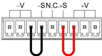
7. If not using local sense, see the remote sense section to wire the sense terminals for remote sensing. Page 70
