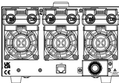
PSW-Multi 3-channel modules with high voltage models.
