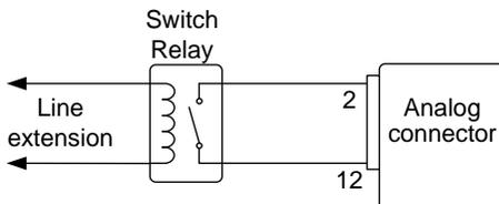
If a single switch control is to be used for Multiple units, please isolate each instrument. This can be achieved by using a relay.
