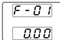
3. Rotate the Voltage knob to change the F setting to F-89 (Show Version).
