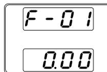
3. Rotate the Voltage knob to change the F setting to F-03 (V-I Mode Slew Rate Select).
