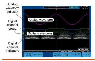
Analog Waveform Used to show the position of the analog waveform Indicator outputs.
