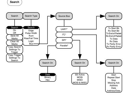
\*The source bus is determined from the bus trigger settings.
