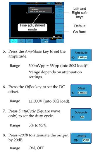
9. The signal will be output immediately from the GEN 1 or GEN 2 outputs.
