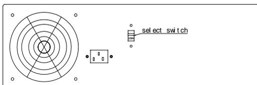
b. The AC input voltage of APS-9102 is fixed either at 115V or 230V. For safety reason, Do not make any change by you own to avoid damaging the instrument.
