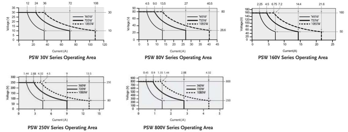
When the power supply is configured that the total output (Current x Voltage output) is less than the rated power output, it functions as a typical Constant Current (C.C) and Constant Voltage (C.V) power supply.
