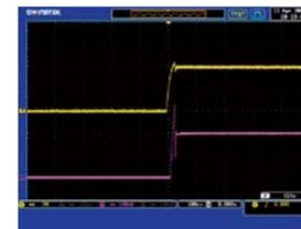
The Inrush Current and Surge Voltage occur at LED Forward Voltage (V<sub>f</sub>) Under C.V Priority
