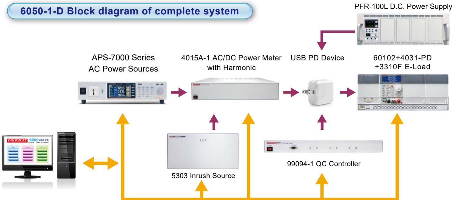
**6050-1-D Single Channel Test System Configuration**
