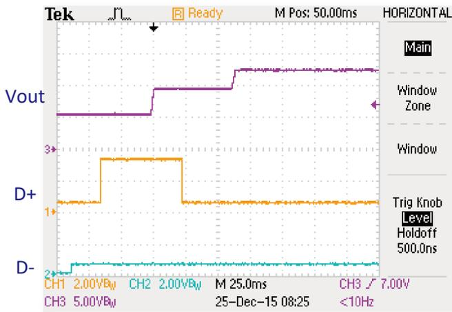
**Transition from 5.0 V to 9.0 V to 12V**
