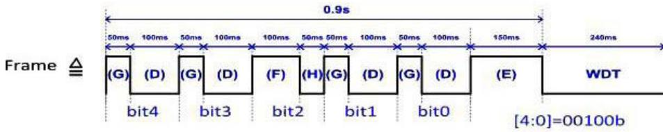
Define the Logic 0 and Logic 1 for bit4~bit0.
