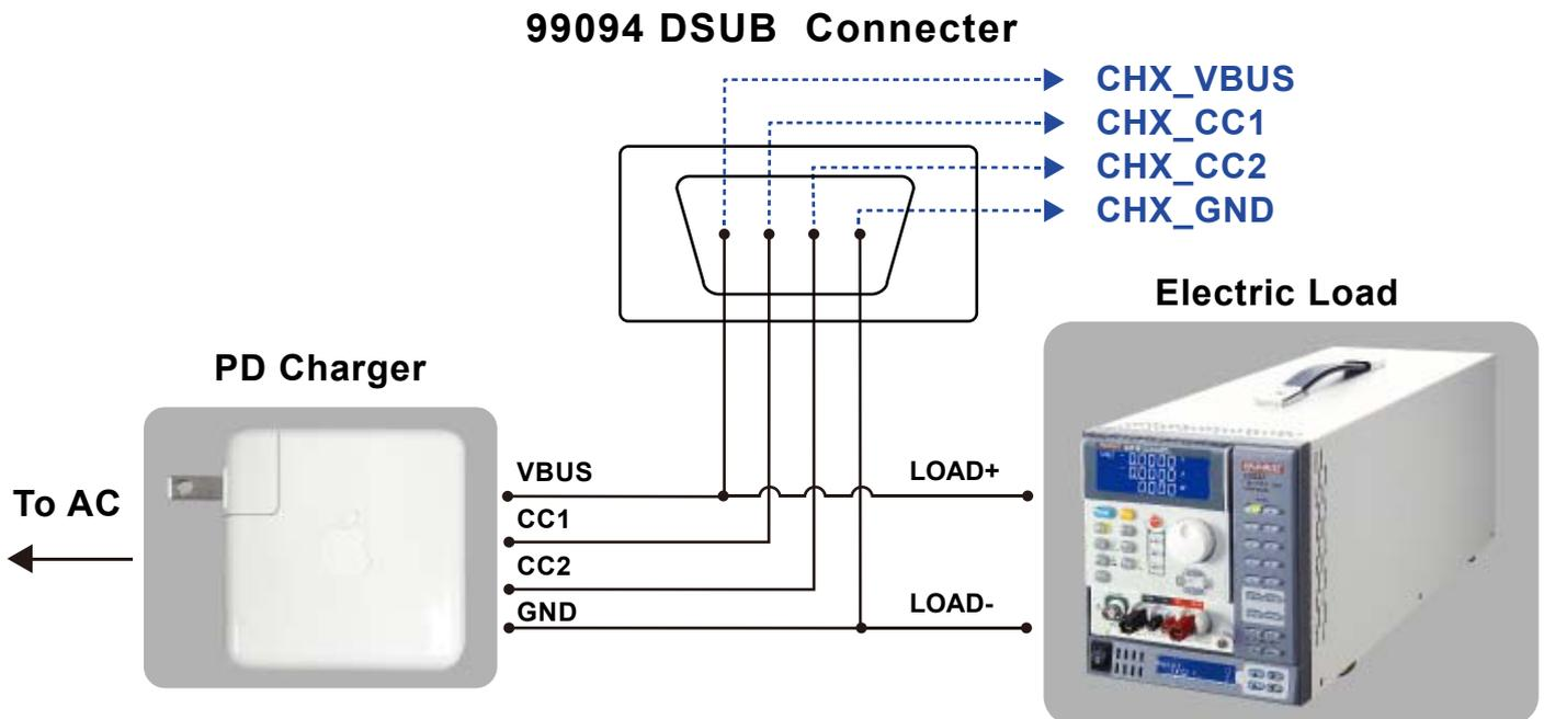
Figure 8 : USB PD Charger Protocol Support
